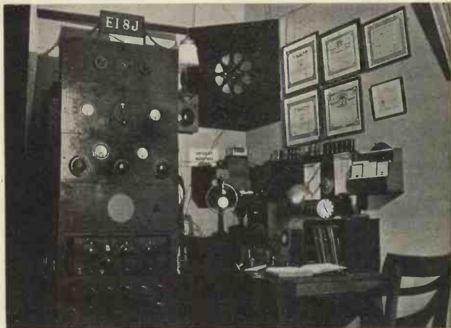
Station EI8J, Dublin. Both receiver and transmitter are accommodated in the rack.
