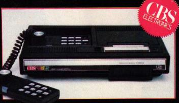
joystick and feature 2 independent fire buttons. The key pad is used for game selection and also for game control with some cartridges. The hand
