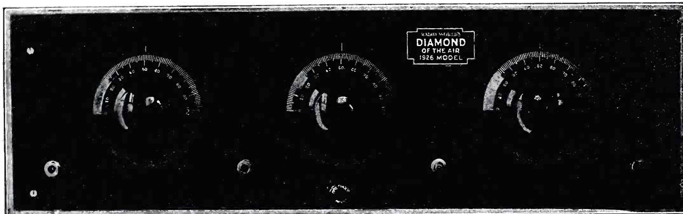
The panel view of the 1926 "Diamond of the Air." The layout of the tuning controls, jacks and battery switch is evenly balanced.
