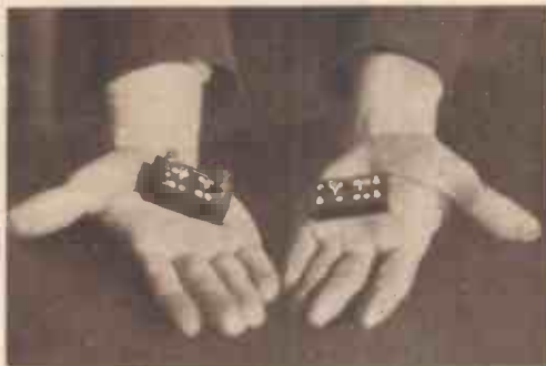
A radio set built on dominoes! These are crystal detectors, but in spite of their midget size, they work on an outside aerial
