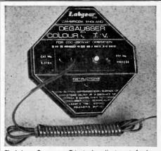
The Labgear Degausser—Prior to the adjustment of colour television receivers, surrounding metal objects should be de-magnetized and the LABGEAR DEGAUSSER Type E.5186 is recommended for this purpose.
