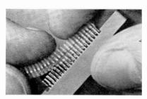
Raychem Thermofit Solder-Pak solder sleeves are supplied in a continuous bandolier. Enough are cut from the strip to terminate one row on a connector. These are then simply slipped onto the terminals of the connector. E162
