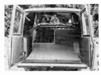
national rental firm. The interior of the vans is lined to the waist with grey padded PVC. The floor is covered with PVC-faced felt. An external rubbing rail and robust tubular steel bumpers are fitted.
