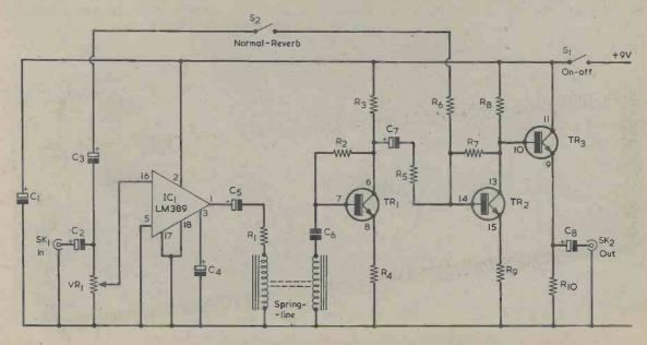
Fig. 1. The circuit of the reverberation unit. The power amplifier and the three transistors are all contained in a single i.c.
