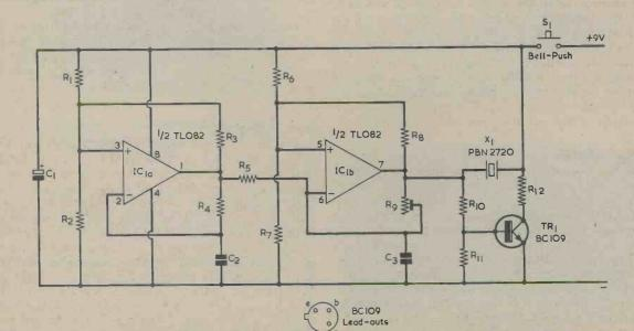
Fig. 2. The circuit of the electronic door buzzer. Low frequency oscillator IC1(a) frequency modulates the audio oscillator, IC1(b)
