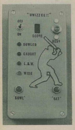
The prototype OWIZZEE! game is housed in a small plastic case with legends on the front panel indicating push-button and l.e.d. functions OWIZZEE is an electronic game designed to simulate a game of cricket, albeit in a simple manner. The game has provided hours of amusement and can be extremely exciting, especially for the youngsters.
