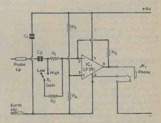
Fig. 1. The circuit of the signal tracer. This is switched on when the earphone plug is inserted into socket JK1.
