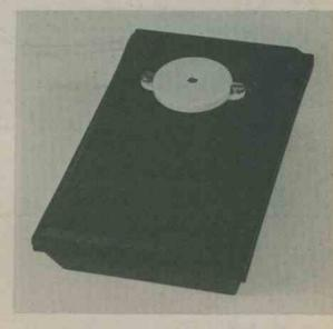
The ceramic transducer is mounted on the front of the case which holds the electronics
