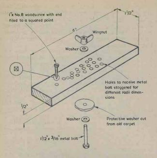
The home-made jig uses readily available parts and can be used to cut clean circular holes in plastic panels. out from an old carpet and a wing nut which fits on the  $1\frac{1}{2}$  in. bolt.
