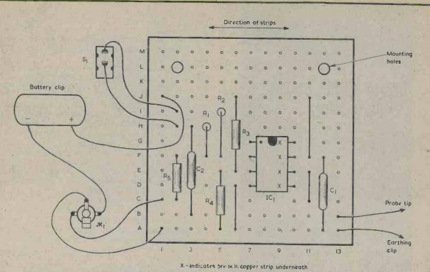
Fig. 3. Layout and wiring on the Veroboard panel. Also shown are the connections external to the panel.
