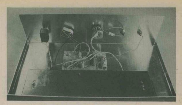
Rear view, illustrating the wiring to the components on the front panel
