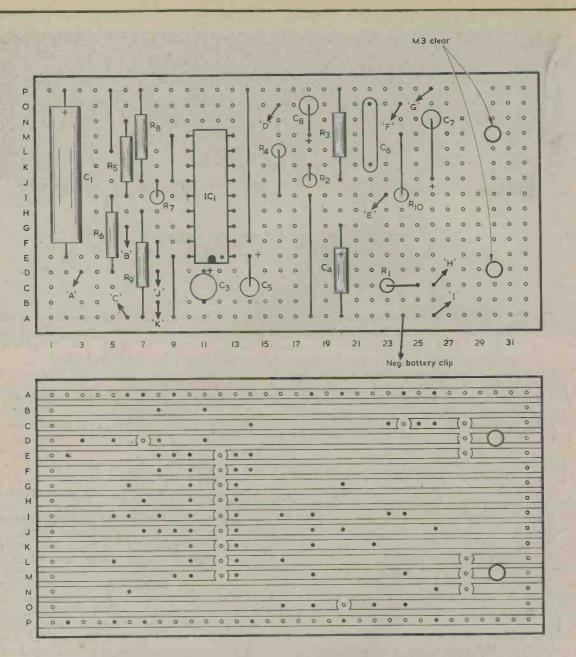
Fig. 2. Nearly all the small components are assembled on a Veroboard of 0.1in! matrix. Component positioning and layout are shown here
