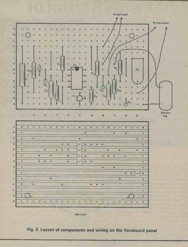
Details are given in Fig. 3. The board has to be cut from a larger size, after which the two mounting holes are drilled. The five breaks in the copper strips are next made, and then the components and link wires are soldered into place. Finally to be connected are the wires to the transducer, the bell-push and the battery clip. The board is secured inside the case by means of two 6BA bolts and nuts, with spacing washers to keep the board underside clear of the inside surface of the case.
