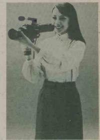
World's smallest home colour video camera, Hitachl's Model VK-C1000 incorporating a single chip MOS colour image sensor.
