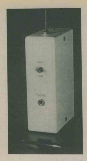
In this view the gain switch S1 is uppermost, with the jack socket below it Note that if the equipment is mains operated, the signal tracer may only be used when the equipment chassis is fully isolated from the mains supply by a double-wound mains power transformer. The tracer must not be used with equipment having a direct connection between chassis and mains because of the risk of a dangerous shock.
