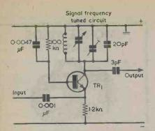
Fig. 5. TR1 in the receiver circuit functions as a common base amplifier at r.f. because of the 0.0047µF capacitor coupling its base to chassis.
