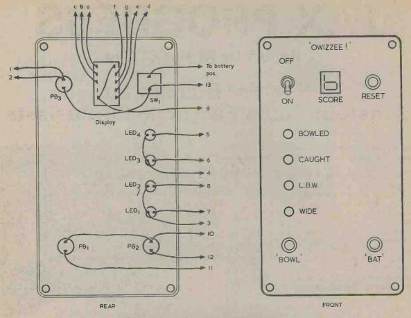
Fig. 3. The wiring and components on the front panel. The numbers from 1 to 13 correspond with those in Fig. 2(b)
