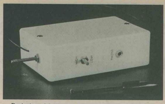
The signal tracer is housed in a small plastic case which can be held in the hand. The probe tip at the end is then applied to the test points in the equipment being checked.
