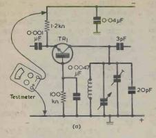
Fig. 6(a). Smithy first checked to ensure that a supply voltage was being passed to the f.m. front-end.
