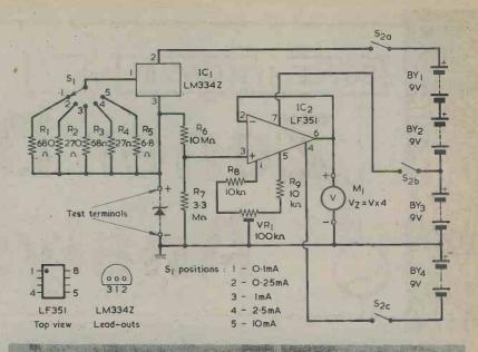
Fig. 2 The circuit of the zener diode analyser. S1 selects five different constant currents which flow through the test diode, the voltage across which is then measured.
