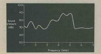
Fig. 1. The output response of the ceramic transducer type PBN-2720
