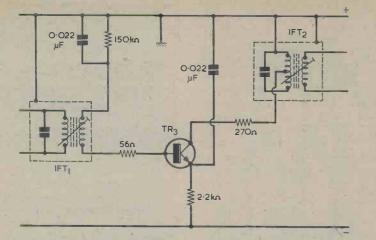
Fig. 2. TR3 is employed in the common emitter mode, as can be clearly seen if the circuit around it is redrawn with the positive supply rail at the top.
