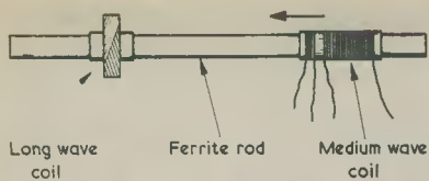
Fig. 1. Smithy brought the receiver serviced by Dick into more accurate alignment by sliding the medium wave coil along the ferrite aerial rod
