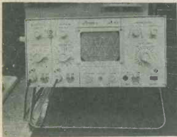
The Scopex 10MHz oscilloscope type 4D-10. This is especially suitable for test, fault-finding and quality control applications in electronics factories
