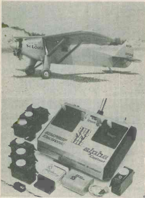
Picture above shows typical plane using the Simprop remote control system powered by General Electric nickel-cadmium batteries. Below, the various elements of the RC system. In the centre: the portable ground unit. Left: the servos. Centre bottom: the receiver and the Simprop power pack using GE Power-Up 15 batteries
