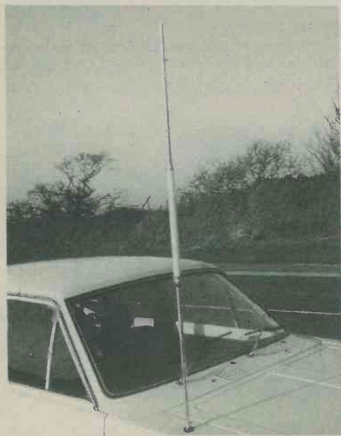
The smart appearance of the Top Band vertical, as fitted to the author's car. It can be readily removed and replaced by a broadcast aerial when not required
