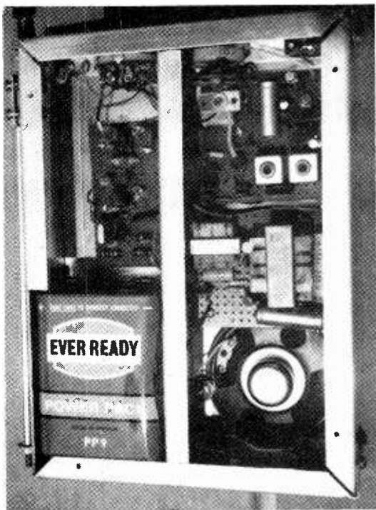
The interior of the transmitter-receiver with all sections mounted in position
