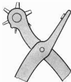
Fig. 5. The upper section of a small leather punch. This may be employed for punching out single Panel-Signs figures
