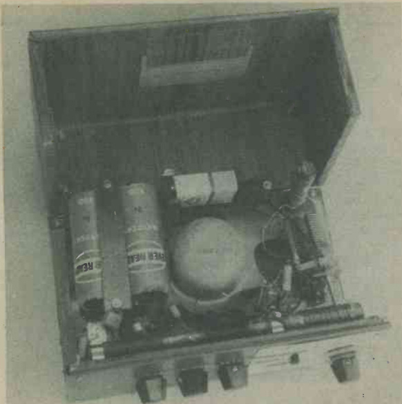
The parts which are visible inside the receiver when the hinged case is opened up
