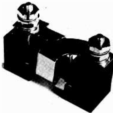
Current sensing relay manufactured by FR Electronics Limited. The unit shown here is intended to monitor heavy currents, and the energising coil has 1 turn only
