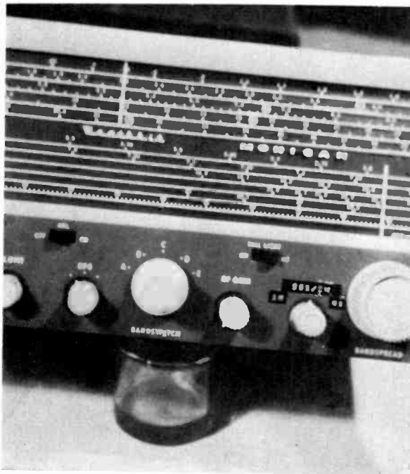
The new function switch, S1, is fitted in place of the panel bush for the aerial trim control
