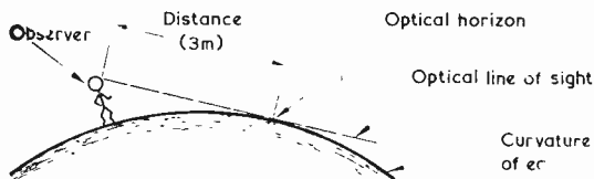
Fig. 1. The optical horizon for a person 5ft. 10in. tall is three miles away
