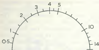
Fig. 4. The Range 1 calibration given with the prototype. Readings are in picofarads
