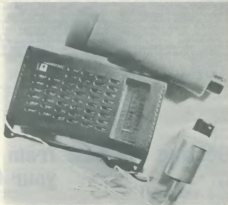
The rechargeable torch of Fig. 1, and the charger of Fig. 2 connected to its radio receiver. Note that both the torch and the radio battery charger are fitted with bayonet mains plugs
