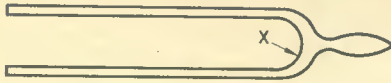
Fig. 2. Small adjustments in tuning fork frequency may be obtained by careful filing at point X
