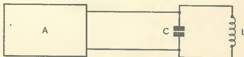
Fig. 1. Illustrating the basic operation of the test unit. Block A is a two-terminal oscillator offering negative resistance to the tuned circuit
