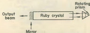
Fig. 13. Q switching with a rotating prism. The prism is shown in the high-Q position
