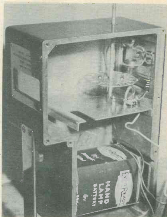
Close-up view, showing the lamp, lens and disc assembly
