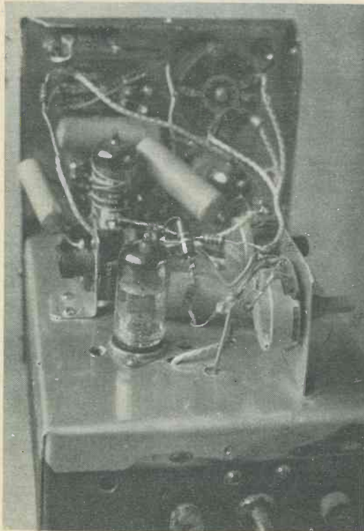
Above-chassis view of the timebase and X amplifier
