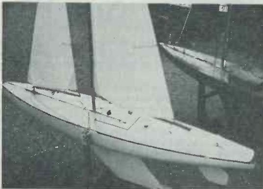
A beautiful model with full control on rudder and sails. The small drum winch controlling the fore and mainsail sheets can be seen in the centre of the deck
