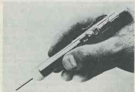
The "Pensource" pocket signal generator that has been produced by Electronic Machine Control Ltd. to provide engineers, radio and TV servicemen with a small and convenient form of input for testing and fault finding
