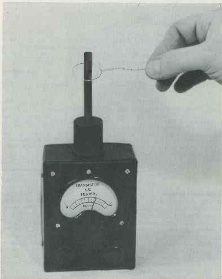
Checking the transistorised shorted turns tester by passing a closed loop of wire over the oscillator core extension. This causes an increase in meter reading. (The unit illustrated here is an experimental model built to the circuit of Fig. 2 but employing a layout differing from that in Figs. 1, 4 and 5)
