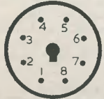
BASE CONNECTIONS FOR THE BRIMAR 3D6.
