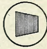
FIG 2 REDUCE MODULATOR INPUT UNTILL A PATTERN SIMILAR TO ABOVE APPEARS ON SCOPE WITH NORMAL SPEAKING VOICE. DISCONNECT MICROPHONE & CONNECT OSCILLATOR ADJUST OSCILLATOR OUTPUT UNTILL SIMILAR PATTERN APPEARS
