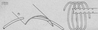
Fig. 2. Showing how acetate spacer strips are threaded on to the coil windings. The coil wire is rotated in a clockwise direction, the ends "picking-up" the holes in the strips as they are reached.
