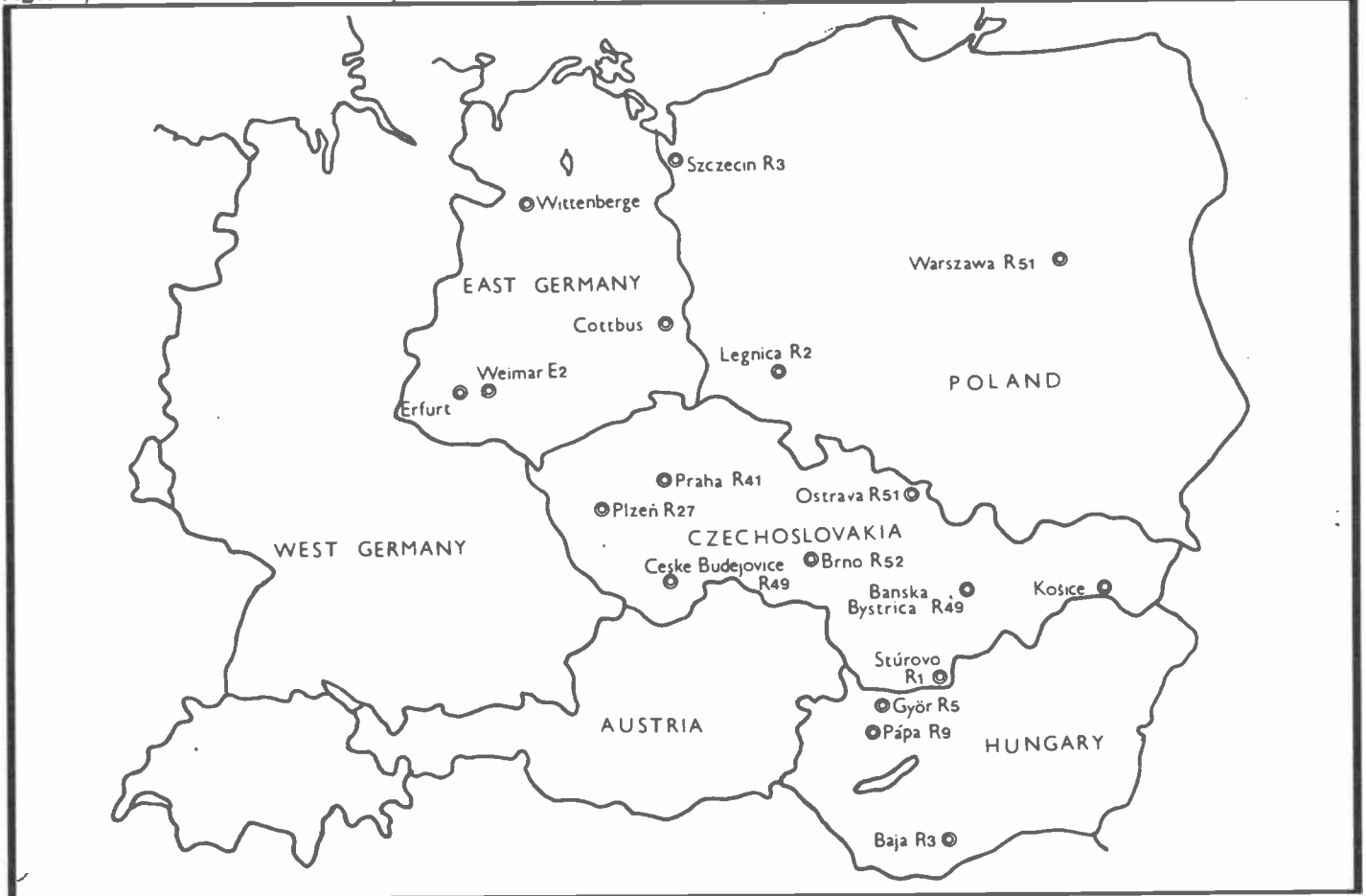
Fig A Map to show distribution of TSS-1 relay transmitters; the reception of which may be possible via sporadic-E or enhanced tropospheric propagation
