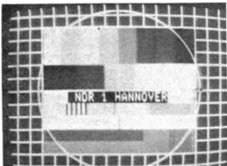
Fig 1 FuBK test card radiated by Norddeutscher Rundfunk in W Germany
