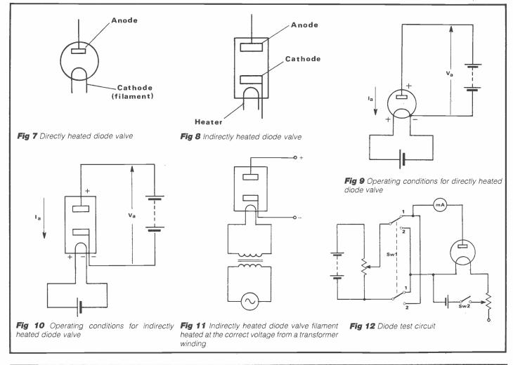
applied voltage (Ohm's Law). This simple state of affairs does not hold true however for a diode, which is a conductor which does not obey Ohm's Law.
