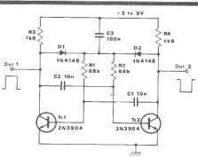
Fig 16 1kHz sure-start astable
