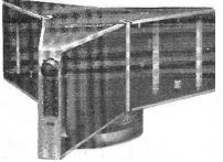
The tests lasted two weeks and were carried out with all the components installed with the exception of the kick motor. After these tests the satellite was due to be 'potted up', that is, everything will be cemented up solid. It then goes back to Germany for final checkout and then out to the Korou launch site for integration and launch, which is now expected to be sometime in October.
