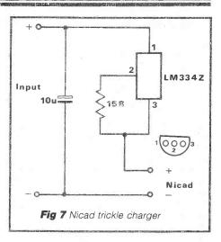
Nicad trickle charger; it will also charge button Nicads well. The output current is set by the formula below:
