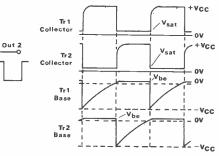
Fig 12 Basic 1kHz astable multivibrator and waveforms
