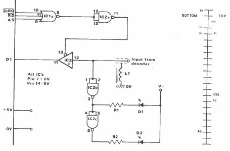
Fig 3 Computer interface circuit
