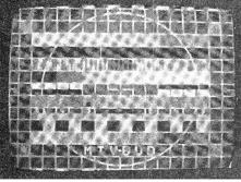
Electronic colour test card radiated occasionally by MTV in Hungary
