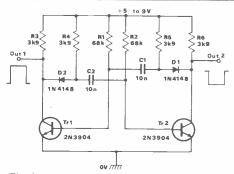
Fig 15 1kHz astable with waveform correction
