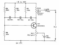
Fig 2 800Hz phase-shift oscillator
