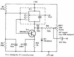
Fig 11 Varicap tuning and FM facility
