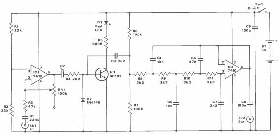
Fig 2 Circuit diagram of the noise limiter
