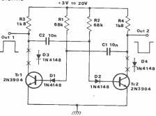
Fig 13 Frequency-corrected multivibrator
