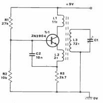
Fig 9 Basic Reinartz oscillator
