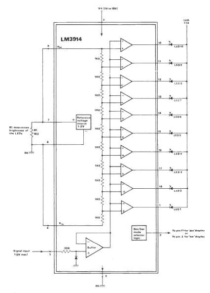
Fig 1 Internal circuit of the LM3914
