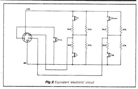
with the 47K resistors forming the 1:1 divider when no switch is pressed. Pushing a switch sends the control voltage high or low through the appropriate 2K2 resistor. It should be noted that the 2K2 value chosen is merely a token value to ensure that there is enough of a swing high or low without a short circuit occurring if two switches are pushed simultaneously.
