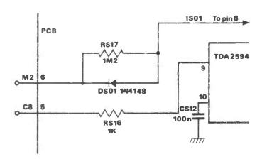
Fla 1 The relevant part of the sync module circuit diagram
