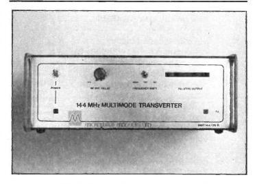
verter. The 28MHz input, of ¼-300mW, is amplified after the RF Vox, ALC control and input level control circuits to an output power of 25 watts.
