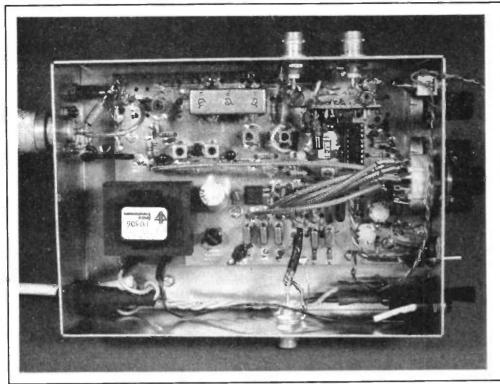
Shows the other receiver – notice the loop around the final multiplier for an external frequency counter. The adjacent BNC connector carries buffered 10.7MHz output for alternative demodulation.
