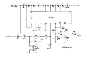
Fig 17 Precision VU meter with low current drain
