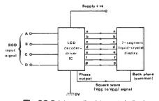
Fig 26 Driving a liquid crystal display
