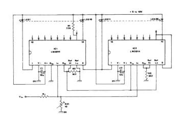
Fig 12 Dot mode 20-LED voltmeter
