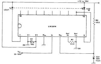
Fig 4 10V fsd meter using an external reference
