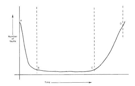
The 'bathtub' serviceability curve. A high initial fault rate at A rapidly subsides due to familiarity with the equipment. From B to C few faults arise and there is little demand for spares. After C faults of age manifest and it is a commercial decision at which point the equipment is replaced.
