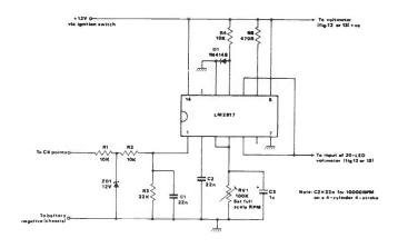
Fig 14 Car tacho conversion circuit
