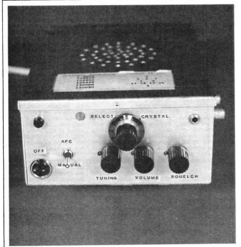
Shows the control panel where the operator can select either AFC or manual tune for any crystal position. Note the reminder sellotaped to the settop of the 'CICADA' group transmit frequencies.
