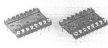
insertion-force collet sockets are used and are available with solder tail or 2- or 3-level wire wrap pins. Collet sockets with gold contacts and gold body or tin body are in a blue Valox low profile body with a notch for polarization or pin identification. 6- through 14pin on 0.500 centres are also available (contact factory for details). For applications requiring a raised socket above the PCB, an elevator type is available (as special) to raise the socket as much as 1.250ins.
