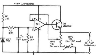
Fig 20 3V to 15V, 0-100 mA stabilised psu
