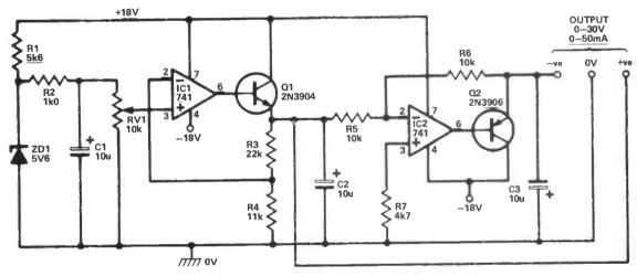
Fig 23 Simple centre-tapped 0-30V psu
