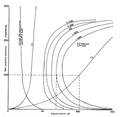
Fig 3 (a) The effect of degree of antenna reactance on the value of C2
