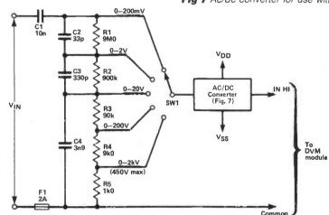
Fig 8 5-range ac volt-meter converter for use with DVM modules
