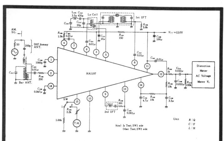
OUTPUT RATIO, SIGNAL-TO-NOISE RATIO, METER SWING AND TOTAL HARMONIC DISTORTION VS. ANTENNA INPUT
