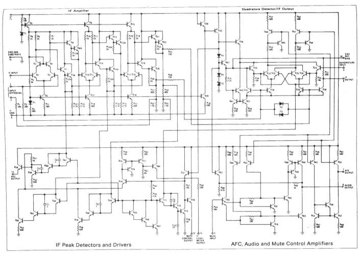
Fig 3 (b) Circuit diagram LM3089
