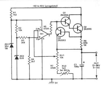
Fig 21 3V to 30V, 0-1 amp stabilised psu
