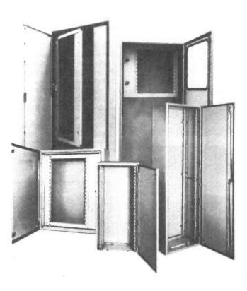
varying in size from 100 x 100 x 50mm to 2-metre-high enclosures which may be built up into suites. Sarel's comprehensive range of enclosures offer degrees of protection from IP 43 (ventilated) to IP 68 (totally dust tight and submersible to 1.8 metre depth).
