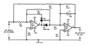
Fig 4 Precision full-wave rectifier
