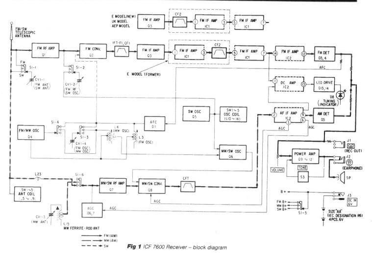
(L3) and the choke on the mixer base, L16. These are quite close on the board layout, and since there is no more direct connection, this must be it! Common emitter mixers require very little drive if delivered via the base, and experience shows that using capacitor coupling can frequently create more problems with the effects of strong signals pulling the oscillator and so forth.
