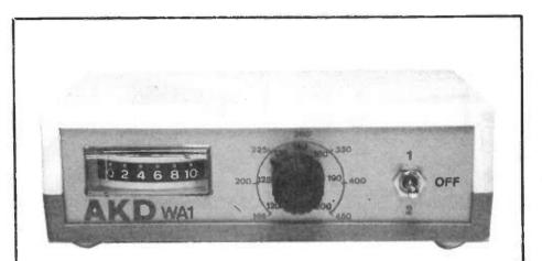
Fig 1 The AKD Wavemeter, Model WA1
