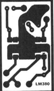
**Fig 2** PCB foil pattern corresponding to Figure 1
