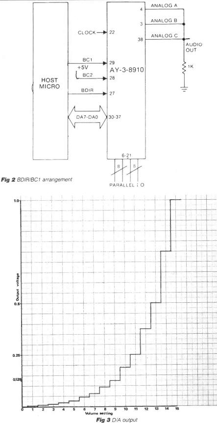
therefore from 30Hz to 100kHz. Because the value set into the register determines the period, rather than the frequency, a conversion table is required in order to determine the 12-bit register value for a particular tone. In Jan 84 a program was published which calculates these values for the chromatic scale.
