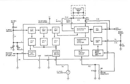
Fig 3 (a) Block diagram LM 3089
