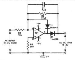
Fig 5 Precision half-wave ac/dc converter
