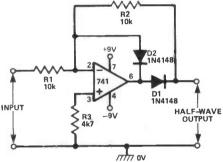
Fig 3 Precision half-wave rectifier
