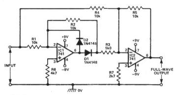
Fig 6 Precision full-wave ac/dc converter
