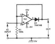
Fig 1 Simple half-wave rectifier circuit
