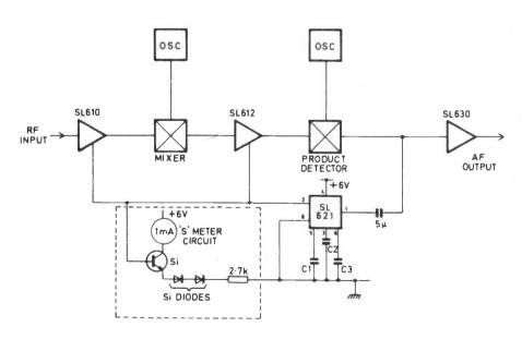
Fig 2 SL621C used to control SSB receiver
