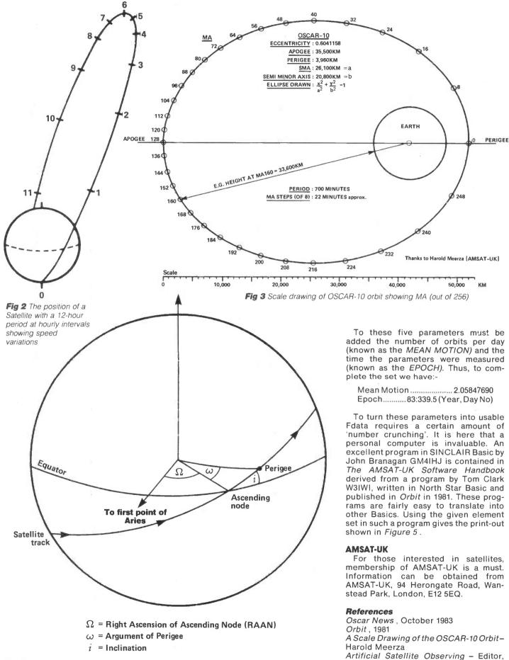
Fig 4 The three elements that fix the orbit relative to Earth
