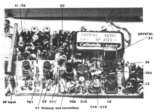
Fig 1 The receiver after modification
