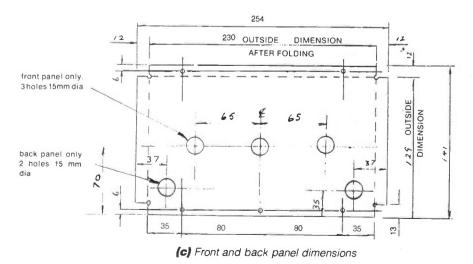
Fig 7 Dimensions of the metalwork
