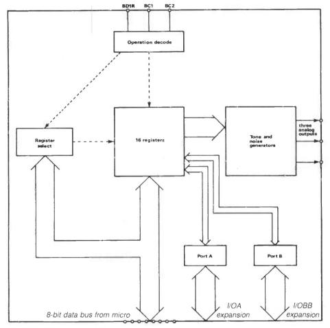
Fig 1 (a) PSG block diagram
