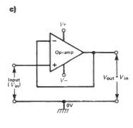
Fig 5 Closed-loop linear amplifier circuits. a) Inverting DC amplifier; b) Non-inverting DC amplifier; and c) Voltage follower
