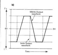
Fig B Effect of slew-rate limiting on the output of an op-amp fed with a square-wave input
