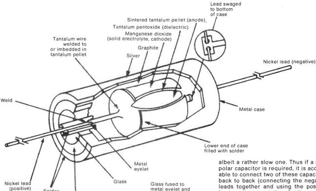
Fig 4 Structure of the metal-cased type of capacitor
