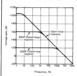
Fig A Typical frequency response curve for the 741 op-amp
