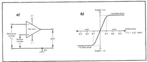
Fig 4 a) Circuit and b) Transfer characteristics of a simple differential voltage comparator
