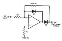
Fig 18 Precision half-wave rectifier
