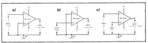
Fig 3 Methods of using an op-amp as a high gain, open-loop, linear amplifier. a) Inverting DC amplifier; b) Non-inverting DC amplifier, and c) Differential DC amplifier
