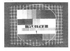
**Fig 1** Finnish second network FuBK test card. (Photograph courtesy of Petri Poeppoenen, Finland)
