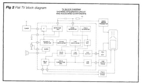
to scan the flat CRT. It runs a check 50 times per second to ensure picture hold'. All coupling, decoupling and phase shift networks are integrated on the chip.
