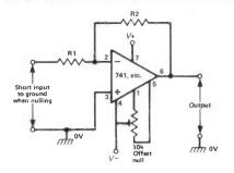
Fig 7 Typical offset nulling system
