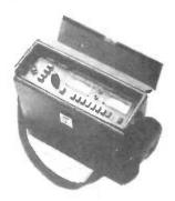
The signals from the aerial are fed to the TC40's  $75\Omega$ coaxial-type input connector, whereupon the meter indicates the RMS voltage and dB's/microvolt on one of seven scales covering 100μV fullscale to 100mV fullscale (lowest reading 20μV). Coarse and fine tuning controls enable Band ITV (45-88MHz), Band II FM (87-108MHz), Band III TV (163 — 230 MHz) and Bands IV and VTV(470-862MHz) to be fully covered. In addition, there are facilities for audio monitoring of AM and FM, and for
