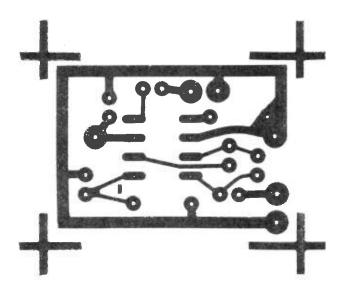
Fig 4 PCB foil pattern for a general purpose audio applications circuit using the SL6270
