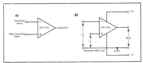
Fig 2 a) Basic symbol and b) Supply connections for an op-amp
