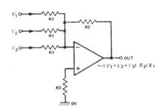
Fig 11 Inverting analogue adder or audio mixer
