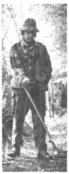
**Photo 2:** The No 4C mine detector. This operates on the induction balance principle and has a 28.5cm search head and solid state electronics
