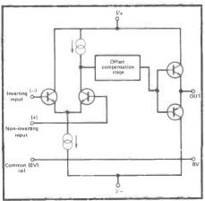
Fig 1 Simplified op-amp equivalent circuit
