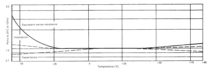
Fig 2 Typical temperature dependence of the characteristics of a 6V plain-foil capacitor
