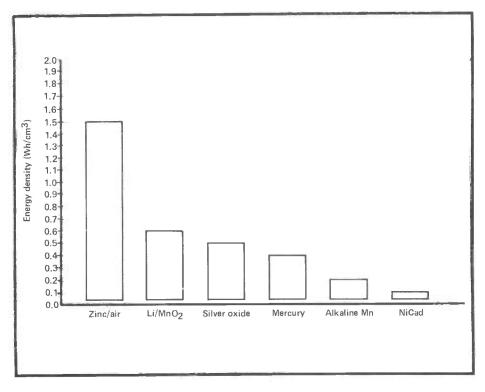
Fig 8 Typical energy densities for a number of battery systems
