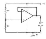
Fig 14 Supply-line splitter
