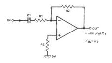
Fig 8 Inverting AC amplifier
