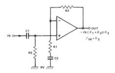
Fig 9 Non-inverting AC amplifier
