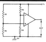
Flg 17 Bridge-balance detector/switch
