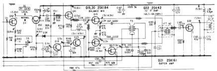
Fig 4 HF input stage of the Sony ICF2001 — an interesting manifestation of the singly balanced FET mixer
