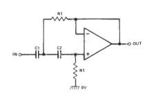
Fig 12 High-pass second-order active filter
