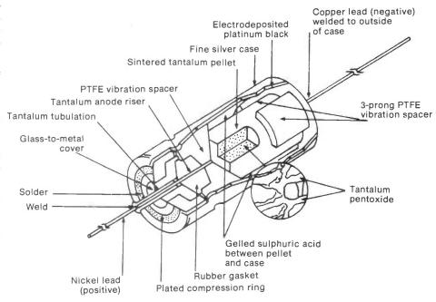
Fig 1 Structure of the gelled type of tantalum capacitor
