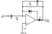
Fig 19 Precision half-wave AC/DC converter
