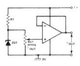
Fig 15 Adjustable voltage reference
