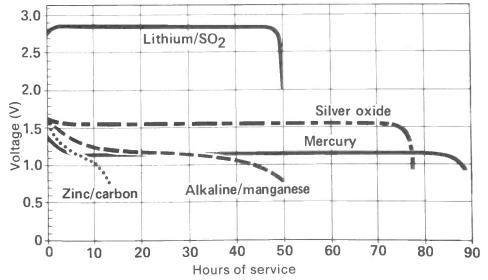
Fig 7 Typical voltage characteristics on medium load of some Durcell batteries
