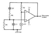
Fig 20 Wien Bridge sine-wave generator
