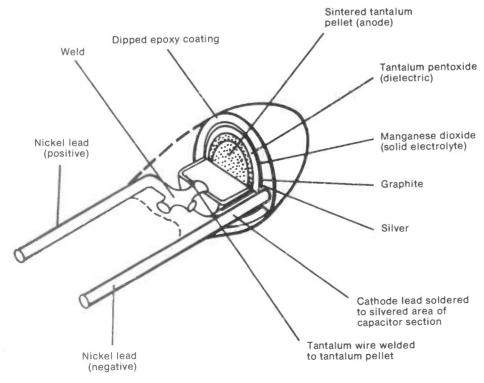
Fig 3 Bead style of tantalum capacitor
