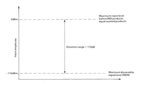
Fig 1 a) Demonstration of why the dynamic range of an amplifying stage is limited by the available voltage swing at the output. b) Receiver dynamic range. NB for **in band** signals, the maximum input level can be considerably greater due to AGC effects.
