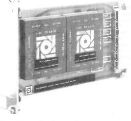
The transformers are prooftested at 5kVac and 120° C, and they conform to IEC 65, BS415 and VDE 0550 regulations.
