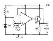
Fig 16 Adjustable voltage power supply
