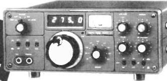
KW + TEN-TEC ARGOSY II HF SSB/CW TRANSCEIVER 10-80 metres, 100 watts (Switchable to 10 watts). Notch Filter. Full break-in on CW. Automatic normal sideband selection plus reverse. 12-14v D.C. input. All solid-state. Excellent for home station, mobile, A WINNER AT LOW COST.
