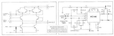
Fig 8 a) Schematic representation and b) Typical modulator circuit for the MC14196
