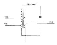
Fig 2: Typical input stage transformation
