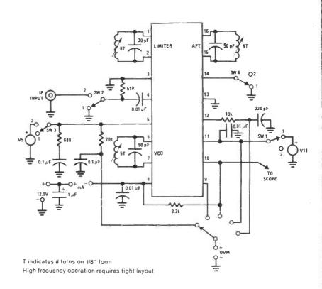
Fig 2: Test circuit
