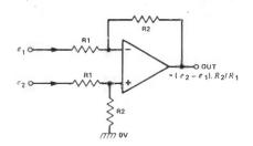
Fig 10 Differential amplifier or analogue subtractor
