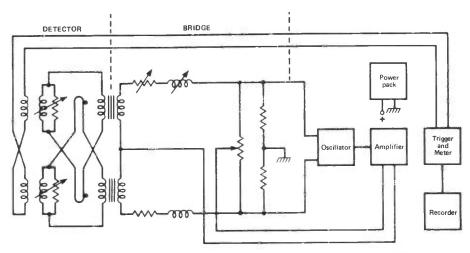
Above ERA Bomb Locator. The mu-metal elements are shown as variable R-L elements
