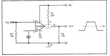
Figure 10. Fast inverting voltage comparator.
