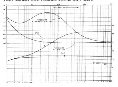
Figure 6. Plot of log gain (dB) against log frequency (Hz) of figure 3.
