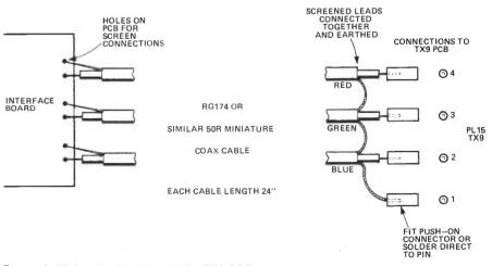
Figure 3. Wiring the interface to the TX9 PCB.
