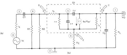
Figure 3. A single transistor amplifier (a) and the linear model (b) which represents it.
