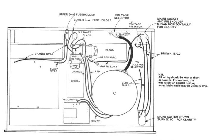
Figure 5: Main amplifier power supply wiring.
