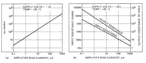
Figure 5. The transconductance (a) and the input and output resistances (b) of the CA3080 vary with the bias current value.
