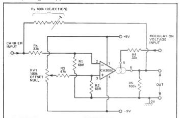
Figure 9. Ring modulator or 4-quadrant multiplier.
