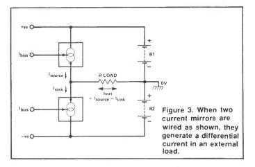
and CMB and fed into the bias and sink terminals (respectively) of CMD, so that the externally available output current of the circuit is equal to  $I_b - I_a$ .
