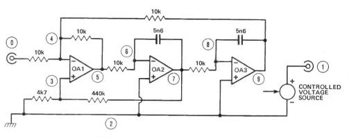
Figure 7. State variable bandpass filter circuit.
