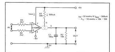
Figure 6. Differential amplifier with 40dB voltage gain.
