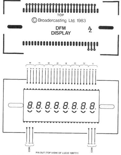
Figure 9. PCB foil pattern (above) and overlay (below) for the 8- digit display.
