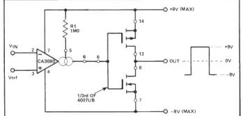
Figure 11. Non-inverting micro-power voltage comparator.
