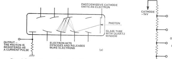
Figure 2. Diagram of a photomultipler (a) and the voltage divider to dynode chain (b) used with it.
