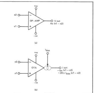
Figure 1. A conventional op-amp (a) is a fixed-gain voltageamplifying device. An OTA (b) is a variable-gain voltage-tocurrent amplifier.
