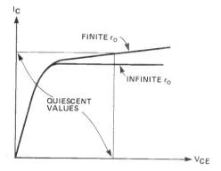
Figure 4. Graph showing the IC/VCE characteristics is modelled by Ro.
