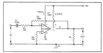
Figure 7. 20dB micro-power inverting amplifier.
