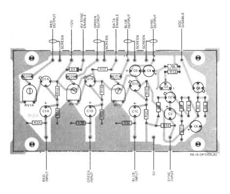
Figure 7a. Component overlay of the completed PCB.
