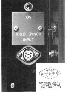
A small panel is fitted below the on/off switch. The inset gives pin designations for the DIN socket.
