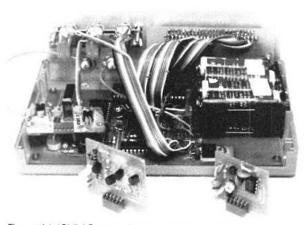
The completed Digital Frequency Meter, as viewed from behind the display. The two boards in the foreground are the 200MHz and 600MHz prescalers.
