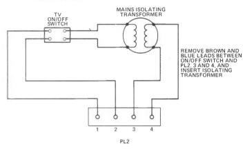
Figure 5. The TV on/off switch can be used to supply the isolating transformer.
