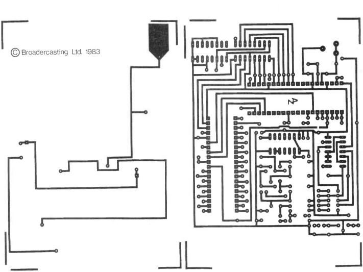
Figure 8b. The two sides of LCD-DFM board (includes pads for 50MHz prescaler).
