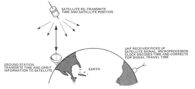
Figure 1. The principle elements involved in satellite time services.
