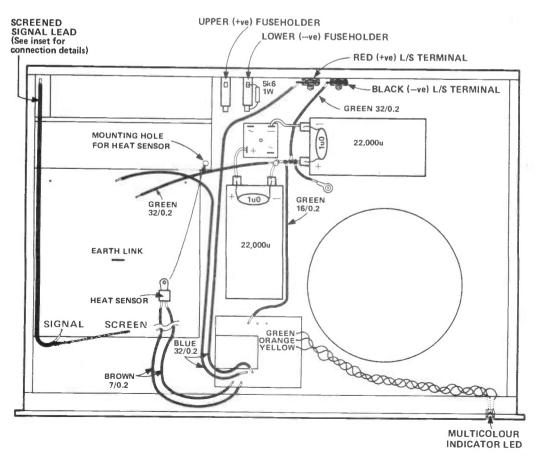
Figure 6: Main amptifier signal wiring.
