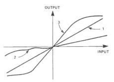
Figure 1. Curves representing the three different component types. Number 1 is for linear components (eg, resistors), number 2 for polarity sensitive components (eg, electrolytic capacitors) and number 3 represents non-linear devices such as op-amps.
