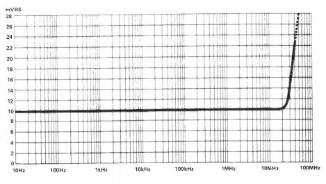
Figure 2: Sensitivity versus frequency-sinusoidal input.
