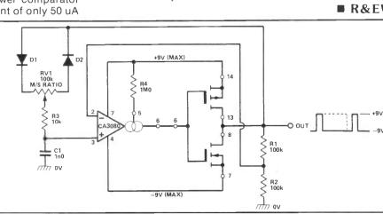
Figure 13. Variable mark-space ratio astable.
