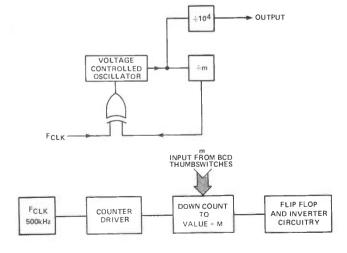
Figure 9. Basic frequency synthesiser and down-counter block.
