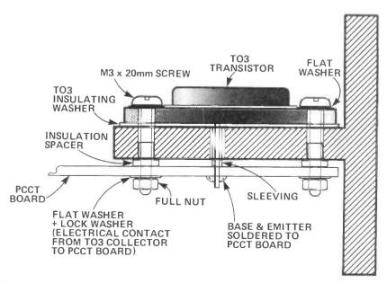
Figure 1: Heatsink bracket section showing power transistor mounting.
