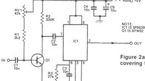
Figure 2a. One of the preamp/prescalers covering the 200MHz range.
