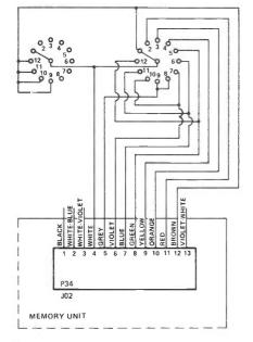
Figure 1: Existing memory switch wiring.
