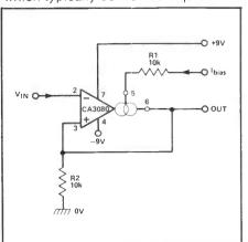
Figure 12. Programmable Schmitt trigger.
