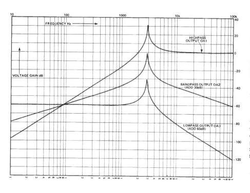
Figure 8. Plot of voltage gain against frequency for the figure 7 circuit.
