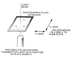
Figure 4. Representation of a scanning densitometer.
