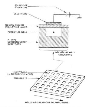
Figure 6. The CCD imaging array, with one cell enlarged to show electrode connections.
