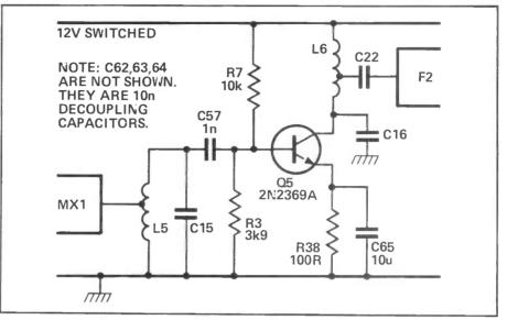
Figure 1: The revised transmit circuit using a bipolar transistor.
