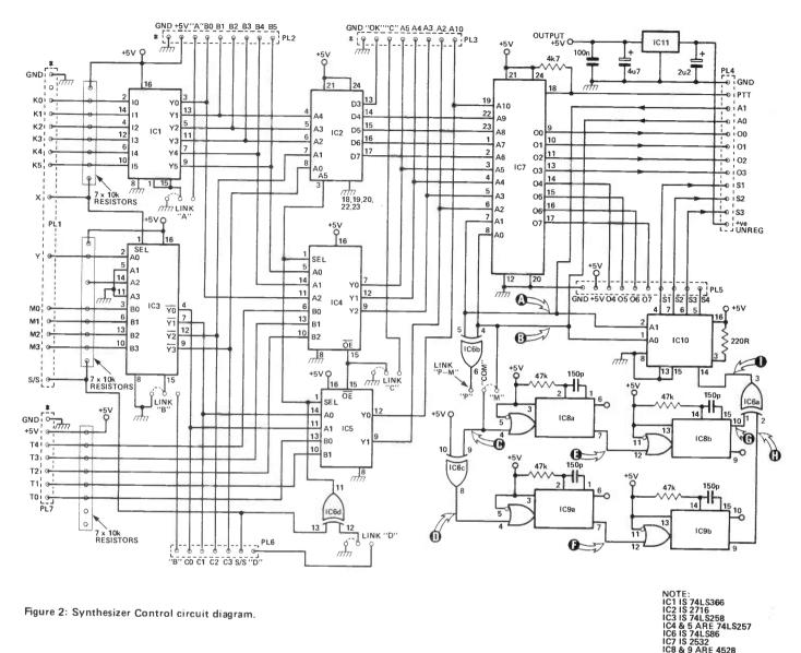
Figure 2: Synthesizer Control circuit diagram.
