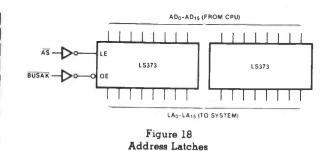
Multiplexing Latched Addresses into  $16K \times 1$  RAMs can be accomplished by synchronizing  $\overline{\text{MREQ}}$  to the CPU clock and then feeding the address bits alternately to the seven chip-address inputs during row (RAS) and column (CAS) address times defined by the circuitry shown below. The 16th address bit is used to select alternate banks of 16K words, if needed, while the lowest bit controls CAS to byte banks within each word bank.
