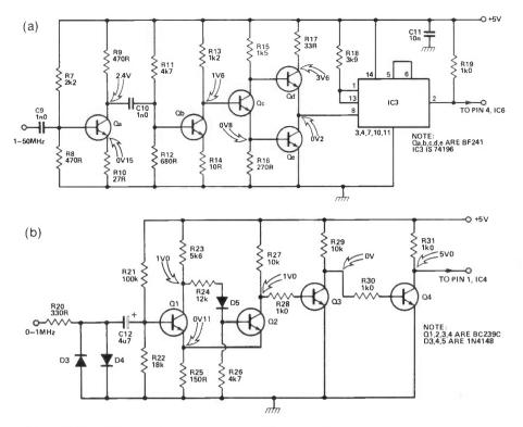
Figure 3. The HF prescaler (a) and LF amplifier (b) which appeared in the November '81 issue of R&EW.
