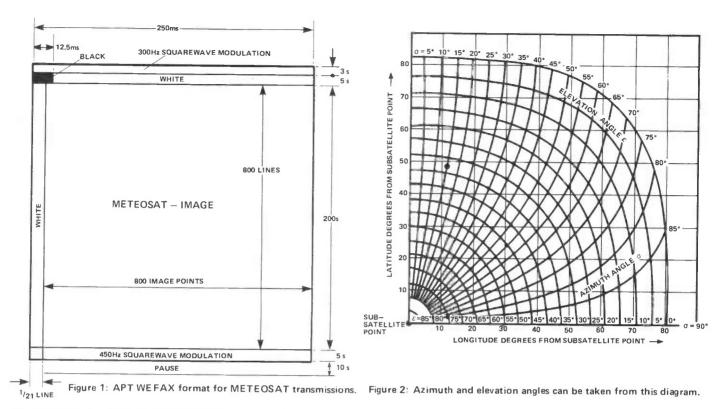
Transmission', which in METEOSAT's case means: 240 lines per minute, 840 pixels per line, 40 of which are in the form of a leading edge (*Fig. 1*). The 300Hz starting tone occurs at the top of the frame in the figure, since the picture will appear from the bottom of the screen and climb up to completion, 800 lines later.
