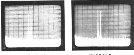
10kHz & 11kHz 85V P/P into 8 ohm
