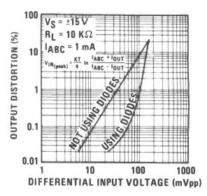
Graph of output distortion vs differential input voltage to show the effect of linearizing diodes.
