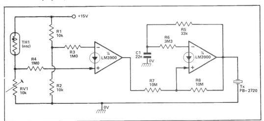
Figure 33: Audible-output over-temperature alarm.
