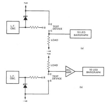
Figure 1. The two basic circuit configurations for testing NPN and PNP transistors.
