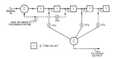
Figure 1. Block diagram of a filter, with feedback path shown by the broken line.
