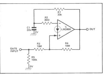
Figure 32: Gated 1 kHz astable.
