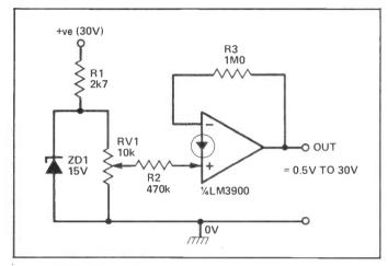
Figure 25: Variable-voltage regulator.
