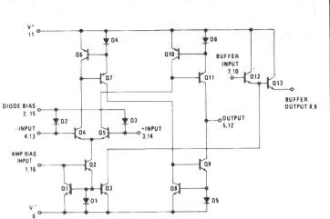
Figure 2: One operational transconductance amplifier.
