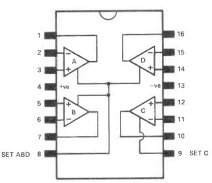
Figure 1: Pin configuration of the LM346N. The layout is identical for the LM124 and LM148.
