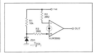
Figure 19: Supply under-voltage detector.
