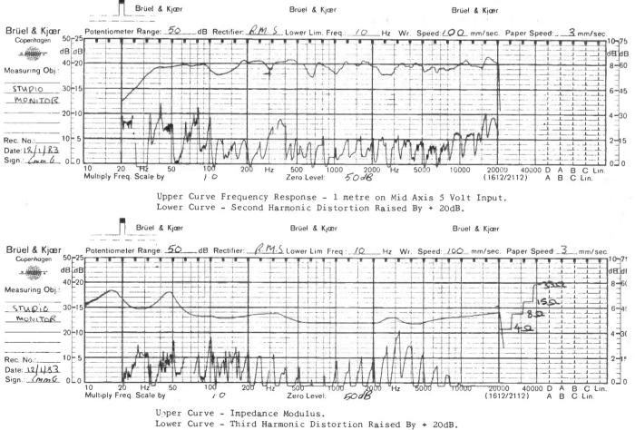
Figure 1: Frequency response, impedance and distortion curves for the Studio Monitors.
