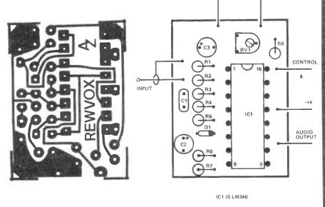
Component overlay and foil pattern for the voice operated switch.
