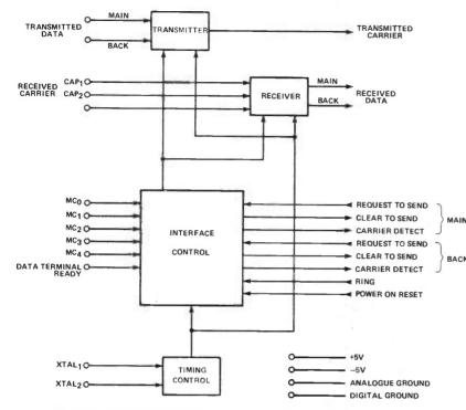
Figure 4. Control circuitry involved in modem design.
