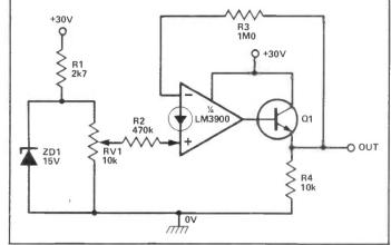
Figure 26: Variable-voltage regulator with boosted output.
