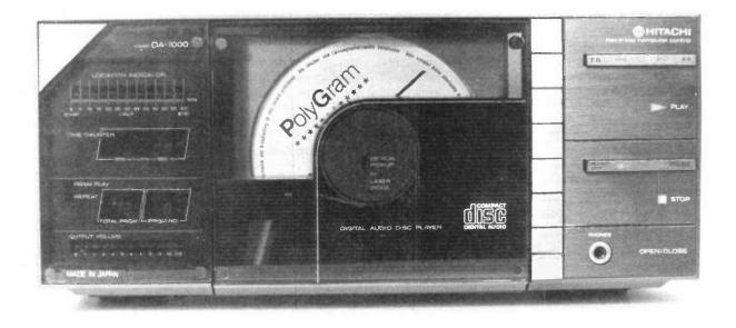
front panel consists of various status and timing indicators while the right hand section is made up of some twelve or so control buttons. These control a range of 'trick' functions and in some peoples' opinion sales of any particular CD player will be determined not so much by the ultimate sound quality, but by the ancillary facilities offered — very much the way of the video market.
