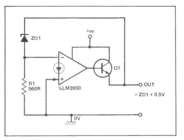
Figure 24: Current-boosted voltage reference.
