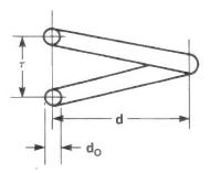
Figure 7: Winding measurements are taken from the mean of the wire diameter.
