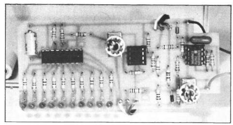
Internal view of the transistor tester.
