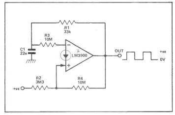
Figure 31: 1 kHz square-wave generator.
