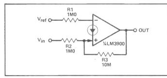
Figure 16: Non-inverting Schmitt trigger.
