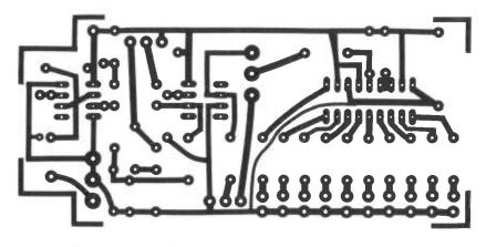
Figure 4. PCB foil pattern for the transistor tester.
