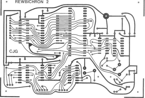
Figure 9. The logic board's foil pattern.
