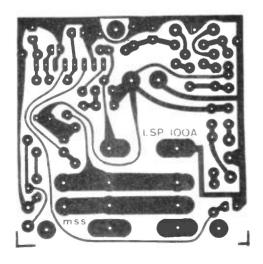
Foil pattern for loudspeaker protection board.
