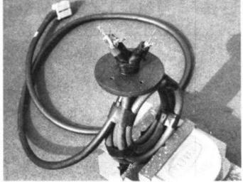
Figure 2. Arrangement of stub and matching sections of coaxial cable and insulating disc for ends of dipoles for the 10 metre crossed dipole antenna.
