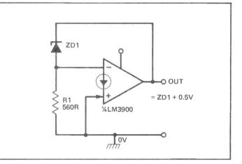
Figure 23: Fixed-voltage reference.
