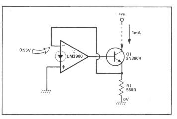
Figure 29: Simple 1 mA current sink.
