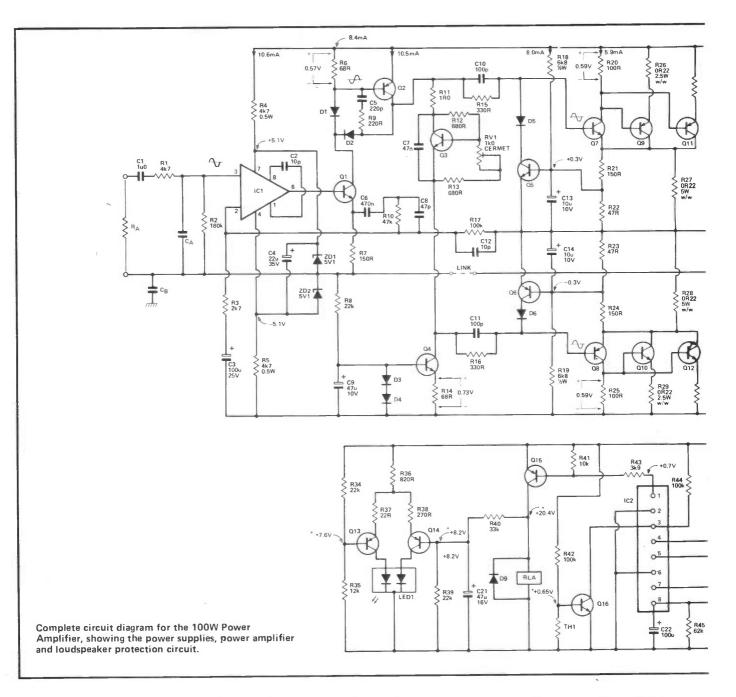
the additional protection provided by supply line fuses FS1 and FS2 one might rightly ask whether the electronic protection circuit is necessary. This can be answered from past experience where amplifiers for repair have been found fitted with brass rods instead of fuses, or the original blown fuse wrapped in silver paper.
