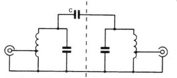
Figure 4: Coupled circuits result in better attenuation while maintaining a reasonable working bandwidth.
