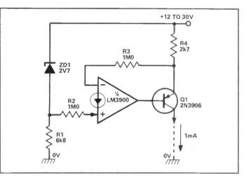
Figure 28: Alternative current source (1 mA).
