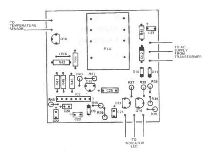
Component overlay for the loudspeaker protection board.
