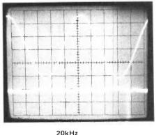
THD of amplifier at 1W into 8 ohm. Distortion trace is amplified by a factor of approximately 750.
