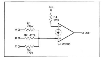
Figure 20: 3-input OR gate (can be converted to a NOR gate by transposing the op-amp inputs).
