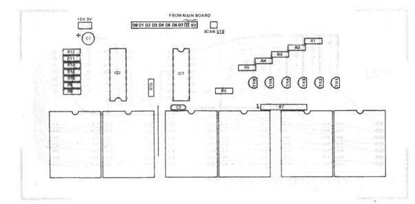
Figure 11. (Above) shows the display board's overlay and Figure 12. (Below) foil pattern.
