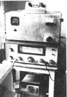
crossed dipole it has Figure 7. The writer's "Satellite Station". given him very many Top — home built 2 metre power amplifier; satellite QSOs indeed. Dne final point. You bottom 2 and 10 metre receiver.
