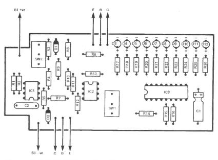
Figure 3. Component placing on the tester PCB.
