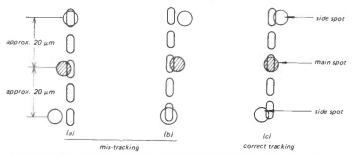
Figure 8: The tracking control system operates by monitoring the amount of light reflected back from the main beam's side spots.
