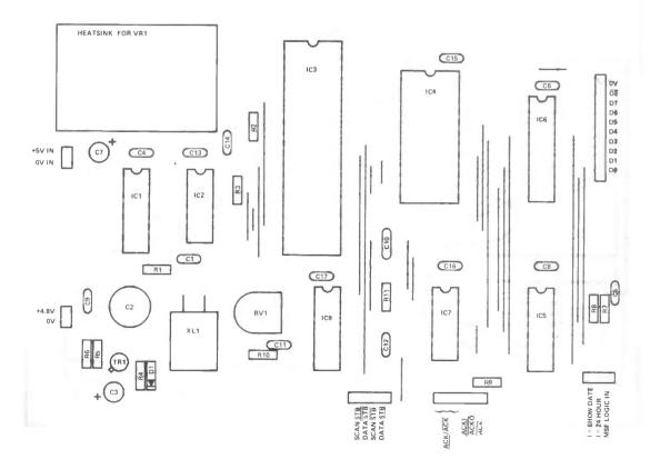
Figure 10. Overlay of the Rewbichron's logic board.
