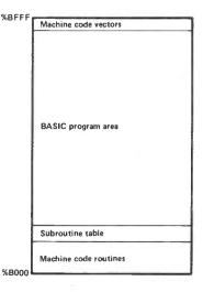
Figure 2. Memory map of Z8 Exec's Part 1 EPROM. This contains the command line interpreter.
