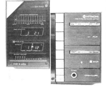
time in minutes and seconds. The volume level can be adjusted by means of an up or down control button its level being displayed by a series of LEDs at the lower left hand side of the player. There's no need to worry about the effect of an electronic attenuator on the quality of the audio signal — the up/down buttons drive a motor that controls an ordinary, passive, pot.
