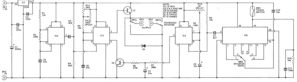
Figure 1: Circuit diagram of the Auto Train Controller.
