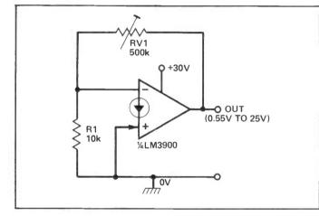
Figure 22: Simple variable-voltage reference.
