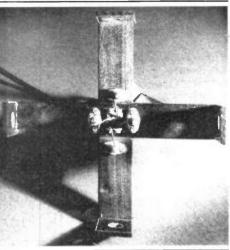
Figure 5. Detail of support inner ends of antenna tubes for 2 metre crossed dipole, showing attachment arrangement to earth mat 'mast', and arrangement of stub and matching section coaxial cables.
