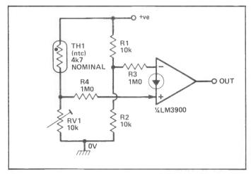
Figure 17: Over-temperature switch.
