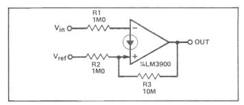
Figure 15: Inverting Schmitt trigger.
