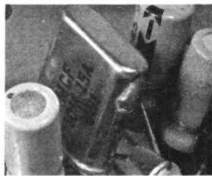
The 10M 15A filter in place. Take care not to short the resistor leads to the can.
