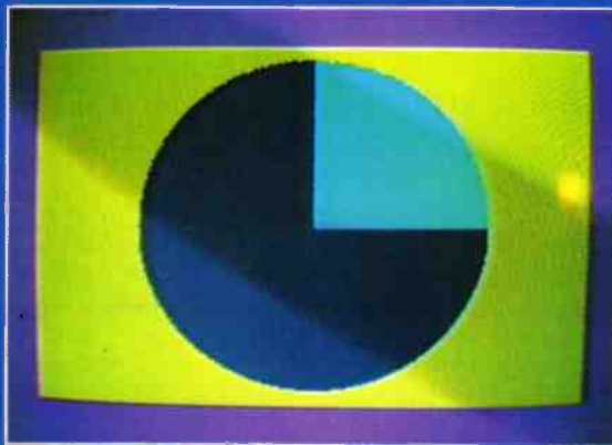
A pie graph with one 90° slice. The centre of the pie was carefully chosen to fall in the bottom left pixel of each character cell.
