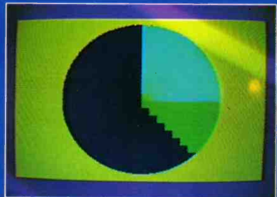
If a slice does not lie on an orthogonal line, the resolution of the pixels is completely obscured by the lesser resolution of the colour.
