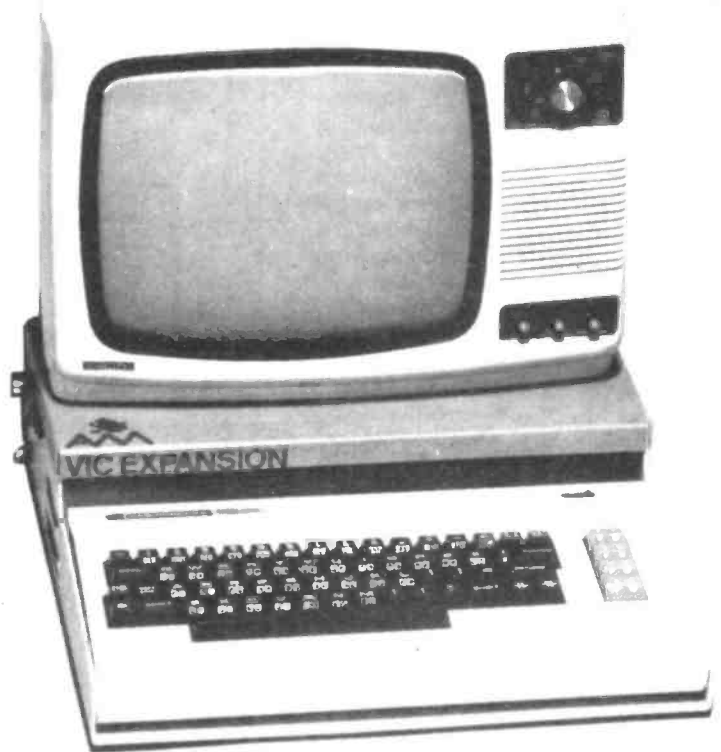
The VIC-20 expansion unit, with lid in place and used as a TV/monitor platform.
