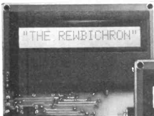
This is the message displayed while the first set of MSF data is being captured, this may take about a minute.
