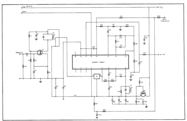
Figure 2: The Ambit 93357 circuit as modified for 455 kHz operation.
