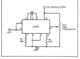
Figure 20: Restricted range VCO, with frequency variable from roughly 72 Hz to 5 kHz via RV1.
