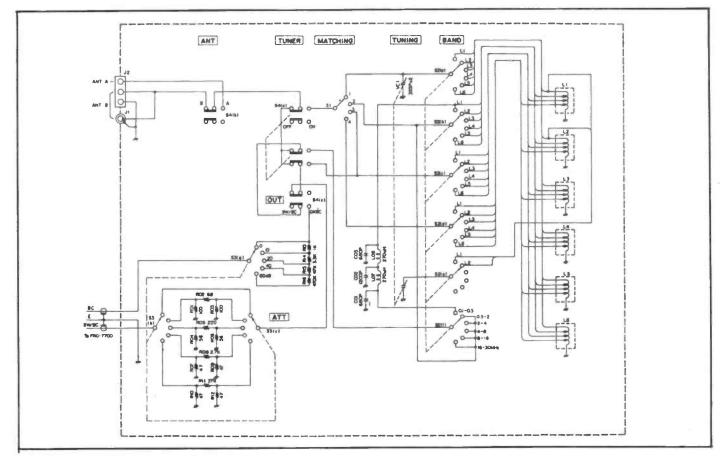
Figure 3: Circuit of the FRT7700 antenna tuner.
