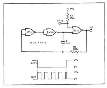
Figure 15: This gated 'ring-of-three' astable is gated by a logic 0 input and has a normally low output.
