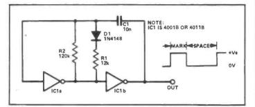
Figure 3: Modifying the astable to give a non-symmetrical output: MARK is controlled by the parallel values of R1 and R2: SPACE is controlled by R2 only.
