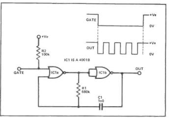
Figure 9: This version of the gated astable has a normally high output and is gated by a low (logic 0) input.
