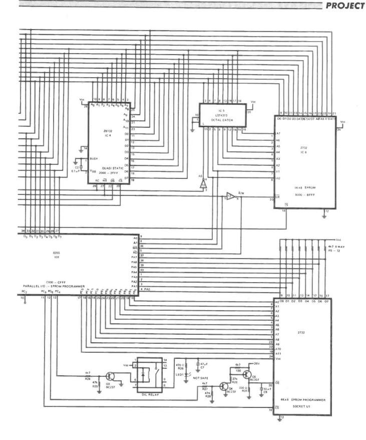
Figure 2: Full Circuit diagram of the Z-8 Tiny BASIC program development system. As can be seen from the photographs the prototype was constructed using wire wrap techniques, but constructors are advised to use the R&EW PCB, or at least take up yoga first!
