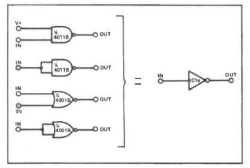
Figure 1b: Ways of connecting a 2-input NAND (4011B) or NOR (4001B) gate for use as an inverter.
