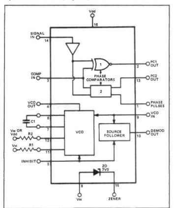
Figure 17: Internal block diagram and pin-outs of the 4046B.
