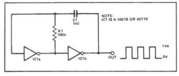
Figure 1a: Circuit of the basic '2-gate' CMOS astable. The circuit operates at 1 kHz with the component values shown.
