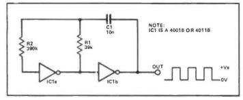
Figure 2: This 'compensated' version of the 1 kHz astable has excellent frequency stability with variations in supply voltage.
