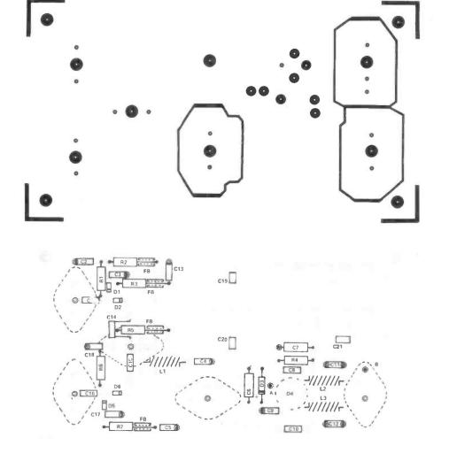
Figure 5: Remote aerial switch, component overlay.
