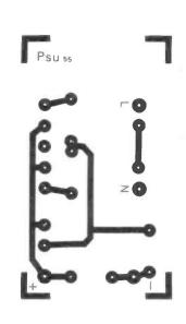
Figure 6: Controller / PSU, foil overlay.
