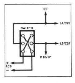
Figure 9: Wiring on rear of switch.
