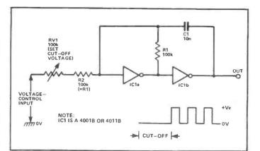
Figure 7: Special-effects VCO which cuts off when  $V_{IN}$  falls below a pre-set value.
