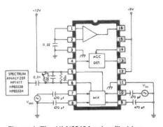
Figure 4: The ULN2243A mixer/limiting IF amplifier.
