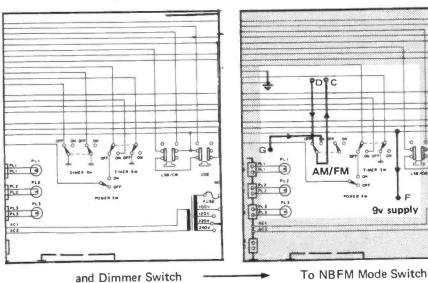
Figure 1: Areas of the R1000 to be modified when fitting the FM facility.
