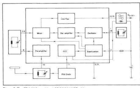
Figure 3: The TDA1062 combined RF/OSC/MIXER chip.
