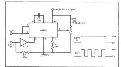
Figure 22: Gated wide-range VCO, using an external gate inverter.
