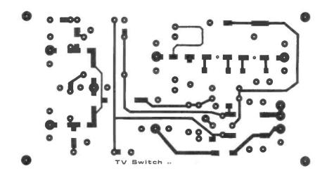
Figure 4: Remote aerial switch, foil pattern - track (component) side above, earth plane (reversed artwork e.g. black = no copper) below.
