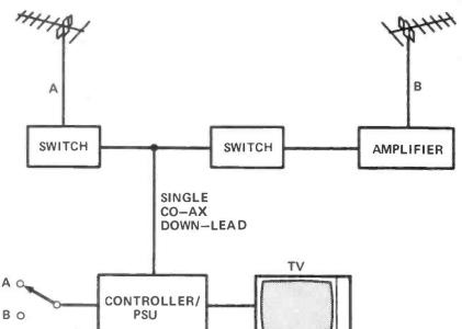
Figure 1: Block diagram of the basic switching arrangement.
