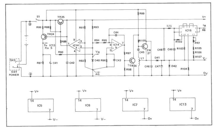
Figure 1: 1503 DMM - Power Supply and Reference Generators.
