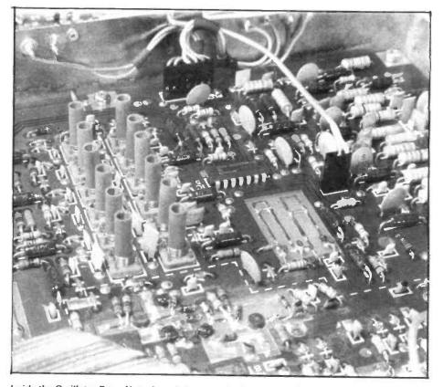
Inside the Oscillator Box - Note the striplines tuned with shorting links
