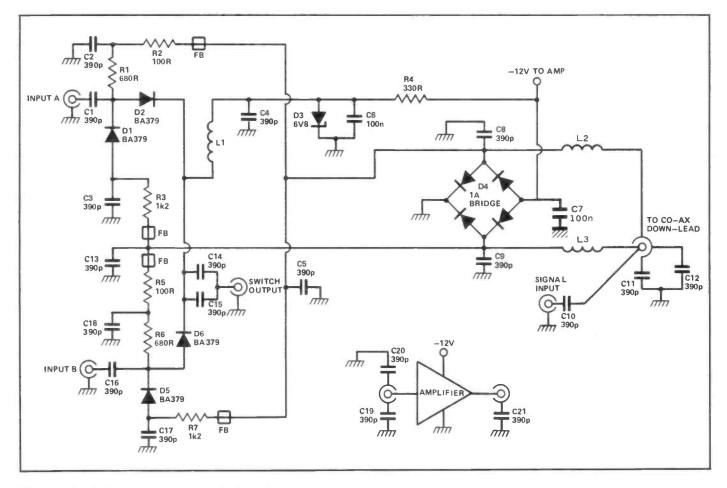
Figure 3: Circuit diagram of the remote Aerial switch.
