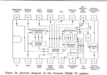
Figure 2a: System diagram of the Ferranti ZN234 TV pattern generator IC.
