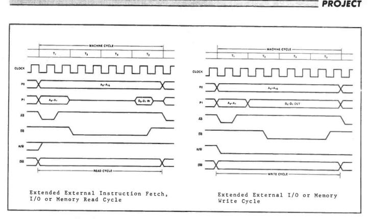
Figure 4: Z-8 bus transactions, showing timing diagrams for external memory read and write.
