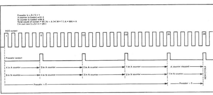
Figure 16: Pulse swallowing.
