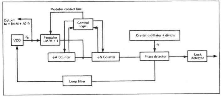
Figure 15: Synthesiser with dual modulus prescaler.
