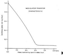
Figure 2d: Transfer characteristics of the UM1286.
