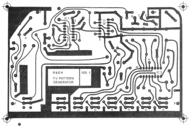
Figure 4: PCB and overlays.
