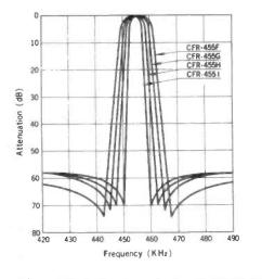
Figure 6: Relative shape factors for low cost 455 kHz ceramic ladder filters.
