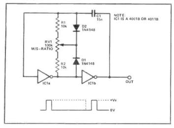
Figure 5: The mark/space ratio of this astable if fully variable from 1:11 to 11:1 via RV1; frequency is almost constant about 1 kHz.
