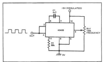
Figure 18: Basic wide-range VCO, spanning near zero to roughly
