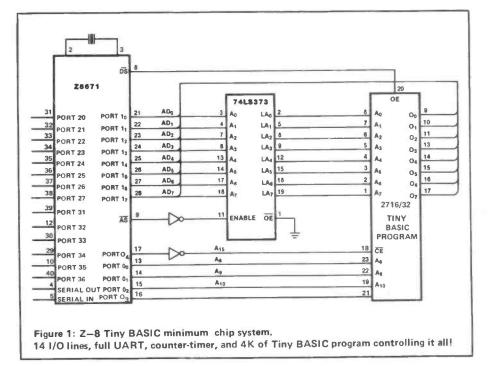
and plugged into a minimum chip Tiny BASIC system, (see Fig 1). Such a controller has 8 bi-directional I/O lines, 3 output only lines, 3 input only lines, two counter timers, and a full duplex UART. Furthermore, it is running Tiny BASIC code held in EPROM, which may easily be modified and maintained via the Z-8 TBPDS.
