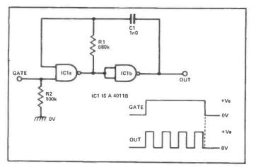
Figure 8: This gated astable has a normally low output and is gated on by a high (logic 1) input.
