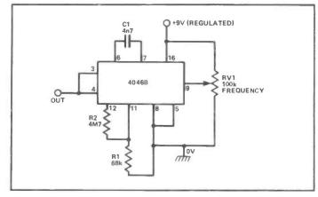
Figure 21: Alternative version of the restricted range VCO:  $f_{max}$  is controlled by C1-R1,  $f_{min}$  by C1 - (R1 + R2).
