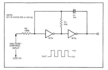
Figure 6: Simple VCO circuit.
