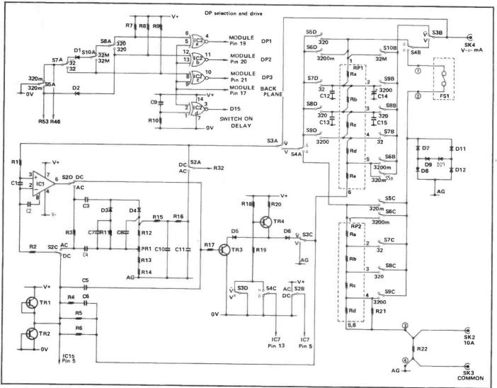
Figure 2: 1503 DMM - Signal Conditioning Circuitry.
