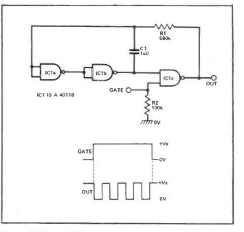
Figure 14: This gated 'ring-of-three' astable is gated by a logic 1 input and has a normally high output.
