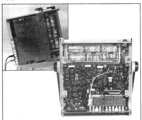
The inside of the 1503 with a view of the electrostatic screen.
