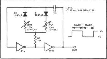
Figure 4: This astable has independently variable MARK and SPACE times.
