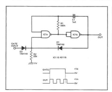
Figure 10: Semi-latching or 'noiseless' gated astable circuit, with logic 1 gate input and normally-zero output.
