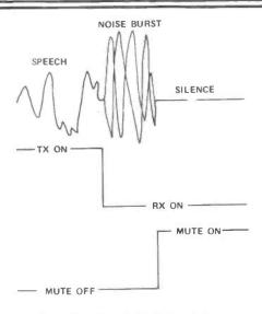
Figure 1: Timing of squelch action between 'overs'.
