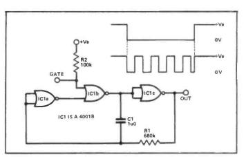
Figure 16: This gated 'ring-of-three' astable is gated by a logic 0 input and has a normally high output.
