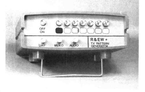
A state-of-the-art piece of test gear generating dot, cross hatch, grey scale and line patterns on Video and UHF outputs. The project incorporates internal/external sound modulation facilities and gives a truly sophisticated performance.
