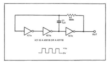
Figure 12: This 'ring-of-three' astable makes an excellent clock generator.
