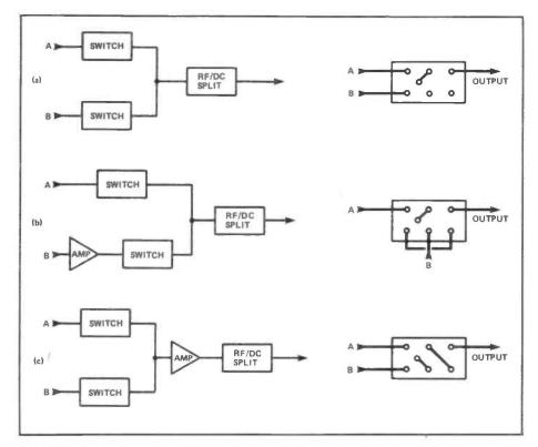
Figure 2: The three possible arrangements of the remote switching unit. The diagrams on the right-hand side show the interconnections on the remote unit for each circuit arrangement.
