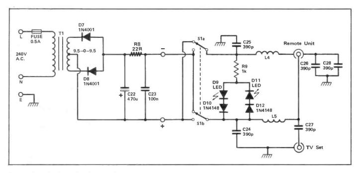
Figure 8: Controller/Power Supply circuit diagram
