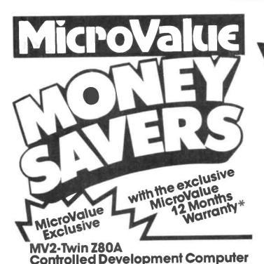
The fully built and tested MV2 microcomputer is controlled by two Z80A microprocessors. Interfaces include R\$232, cassette, 2 x 8 bit parallel ports, and graphics including programmable graphics. It provides  $80 \times 25$  screen format and includes 64K RAM, Integral PSU
