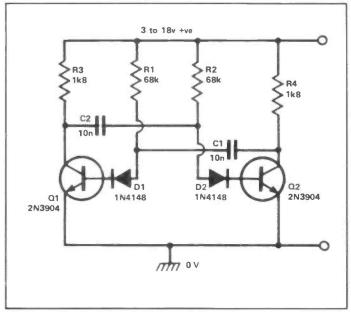
Figure 2: This version of the 1kHz astable has frequency correction applied via D1 and D2 and can be used with any supply voltage up to the breakdown limits of the transistors.
