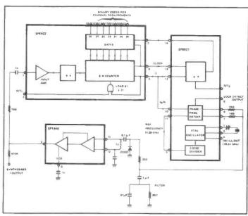
Figure 11: Plessey CB synthesiser - Block diagram.
