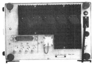
Rear view of the TR4122B. Note the X,Y and Z output sockets.
