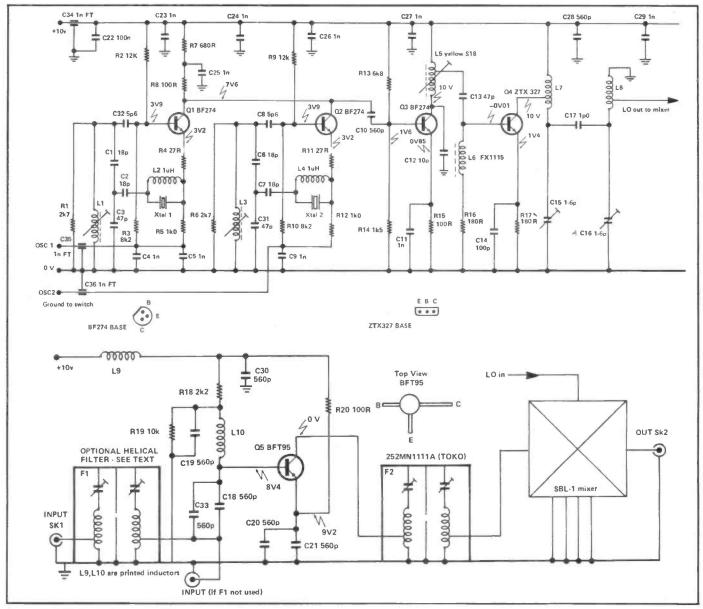
Figure 2: Full circuit diagram of the converter.
