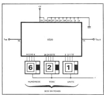
Figure 8: A single I.C. programmable counter with a - 3 to - 999 capability.
