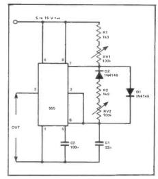
Figure 13: Astable with mark and space periods independently variable over the approximate range 15uS to 1.5mS.
