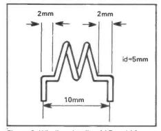
Figure 3: Winding details of L7 and L8.
