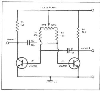
Figure 5a: Basic variable M/S ratio astable, operating at about 1100Hz.
