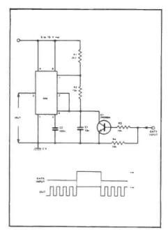
Figure 16: Electronically gated astable, with the gate signal applied to C1 via Q1.
