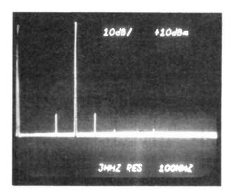
Analyser photo' showing the excellent output purity of the local oscillator; all spurious is greater than 46 dB down on the wanted signal, Centre frequency is 490 MHz, horizontal = 100 MHz/div, vertical = 10 dB/div.
