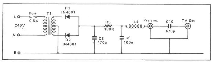
Figure 1b: The PSU circuit diagram.
