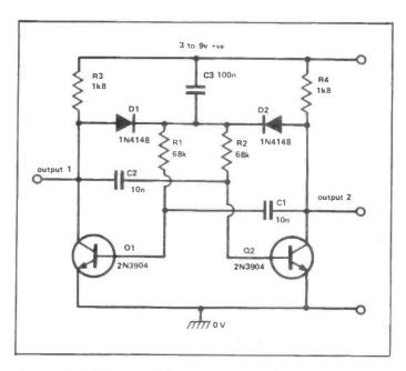
Figure 4: This 1kHz astable has a sure start facility.
