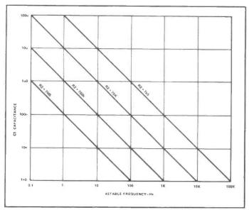
Figure 10b: Approximate relationship between C1, R2 and frequency of the 555 astable when R2 is large relative to R1.
