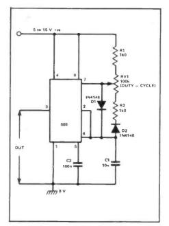
Figure 14: Astable with duty cycle variable from 1% to 99% via RV1. Frequency is almost constant at 1.2kHz.
