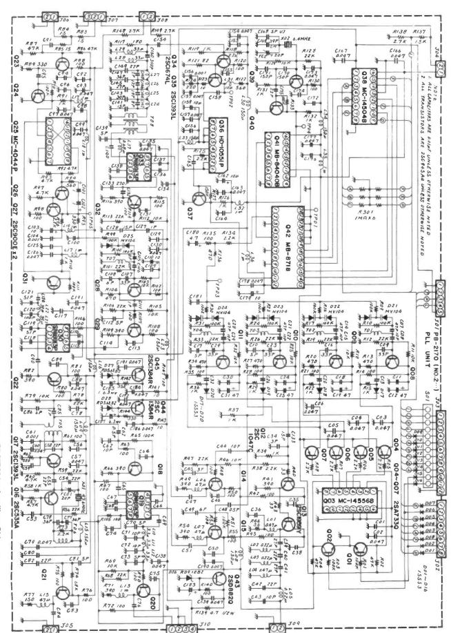
Fig. 4a: FRG7700 local oscillator PLL system
