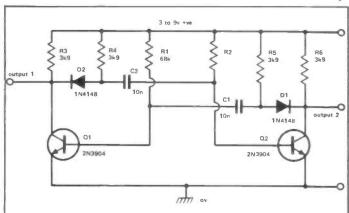
Figure 3: This version of the 1kHz astable has waveform correction applied via D1 and D2 and produces excellent square waves.
