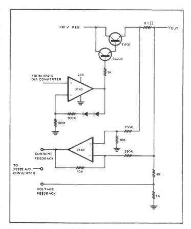
Figure 4: Programmable 0-25 V 1 Amp PSU.
