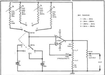
Figure 8: Four-decade (2Hz to 20kHz) square wave generator. The preset pots enable the circuit to use a single calibrated frequency scale.
