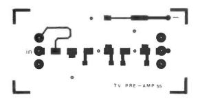
Figure 2: Pre-amp PCB foil pattern (top side). The lower side of this double-sided board is unetched and used as an earth plane.
