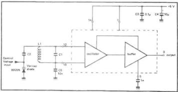
Figure 4: Application of MC1648 as a VCO and Buffer.
