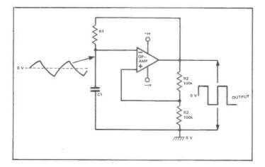
Figure 6: Basic op-amp relaxation oscillator circuit.
