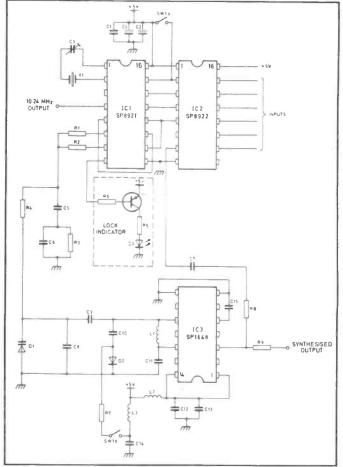
Figure 12: Plessey CB synthesiser - circuit diagram.
