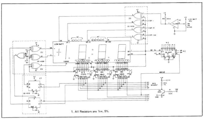
Figure 3: Circuit diagram of the display board of the 2015A DMM.
