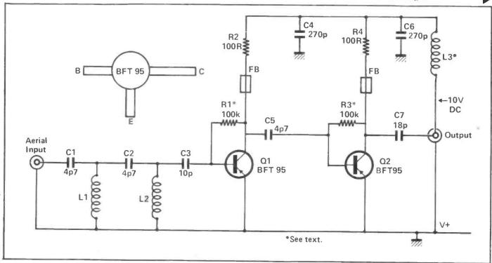
Figure 1a: The TV pre-amp circuit diagram.
