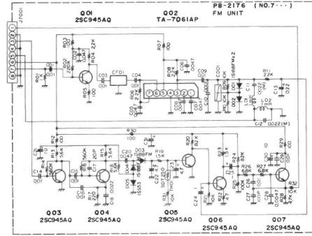
Fig. 1: The NBFM demodulator.
