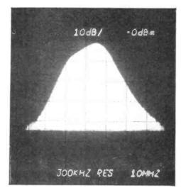
Bandpass response of converter (fitted with both helical filters). Centre frequency 430 MHz, 10 MHz/division horizontal; 10 dB/division vertical.
