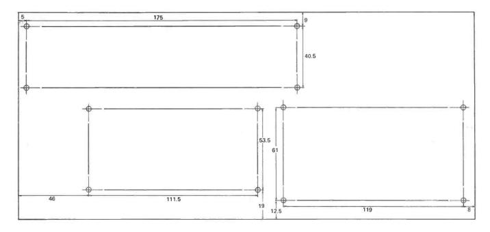
Figure 19: Constructional details of the bottom panel (viewed from the non-coated side).
