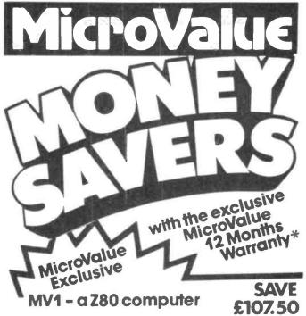
The MV1 computer kit uses the ubiquitous Nascom 1 Pcb and the Z80 CPU. Interfaces are included for television, printer and cassette. 2K memory, Gemini power supply (drives up to 3 extra boards). Cherry full ASCII keyboard and Quantum Graphics are also included. Available with either an ASCII version of the
