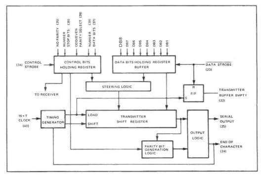
Figure 3: Block diagram of the UART transmitter.
