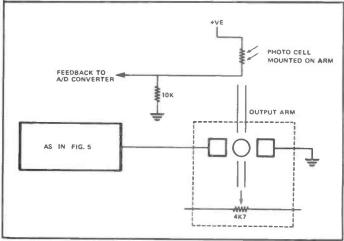
Figure 6: Simple computer controlled light-seeking robot.
