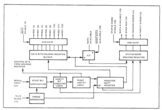
Figure 1: Block diagram of the receiver logic fo the AY-5-1012 UART.
