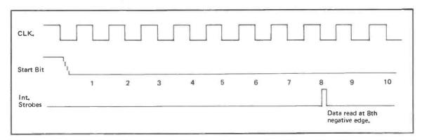
Figure 2: Waveforms demonstrating the receiver's window sampling technique.
