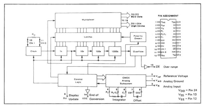
Figure 1: Block diagram of the basic DMM circultry, together with pin assignments of the MC14433 A/D converter.
