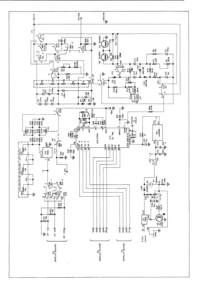
Figure 2: Circuit diagram of the main board of the 2015A DMM.
