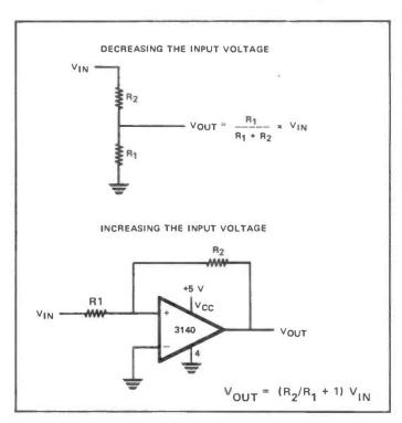
Figure 1: Input scaling methods.
