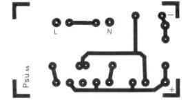
Figure 4: PSU PCB foil pattern.
