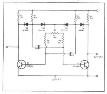
Figure 5b: This improved version of the variable M/S ratio astable has waveform correction and the sure start facility.
