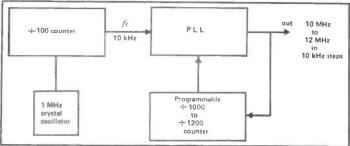
Figure 3: Basic Form of a PLL Frequency Synthesiser.
