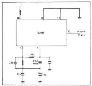
Figure 5: A Reference Oscillator/Divider in One Chip.
