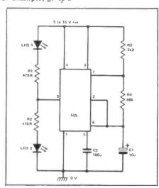
Figure 12: This 2-LED flasher operates at just under 1Hz. One LED turns on as the other turns off, and vice versa.
