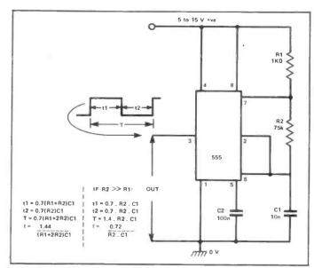
Figure 10a: Basic circuit of 1kHz '555' astable, with timing formulae.
