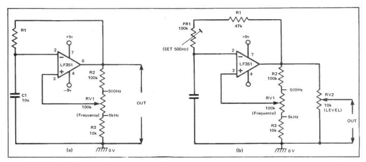
Figure 7a: Simple 500Hz to 5kHz square wave generator, and Figure 7b: an improved version of the circuit.
