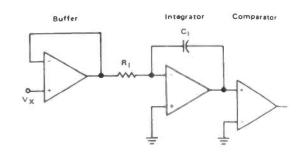
Figure 5: Equivalent circuit diagrams of the analogue section.
