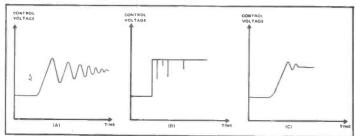
Figure 10: Effects of loop filter on VCO Control voltage.
