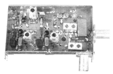
Two for the price of one: a sophisticated full coverage 70 cms to 2 m converter, plus a channel - 52 TV output for receiving and viewing.
