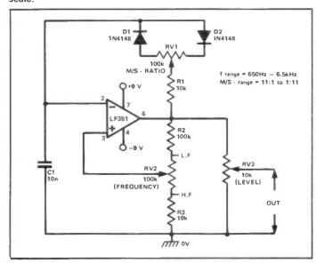
Figure 9: Variable frequency, variable mark/space ratio 'square wave' generator.
