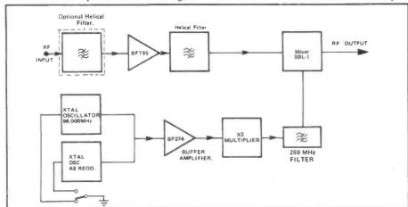
Figure 1: Block diagram of the converter system.
