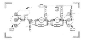
Figure 3: Pre-amp overlay Note that components are assembled on the top track side.
