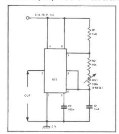
Figure 11: This variable frequency square wave generator covers the range 1.4kHz to 15kHz via RV1.
