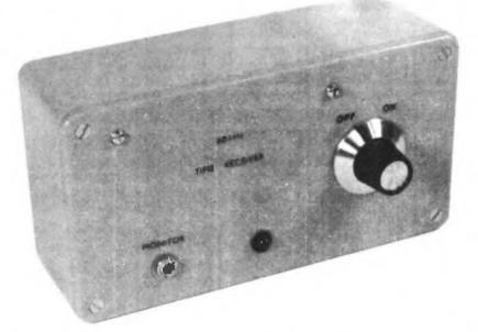
1. The 60kHz Time Receiver built into a plastic box, showing the audio and visual monitors and the on-off switch.
