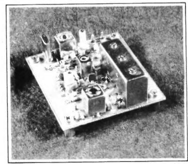
The completed converter PCB
