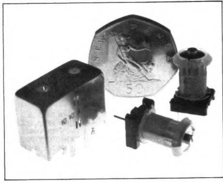
An 'undone' view of the 2 pole version of the helical filter
