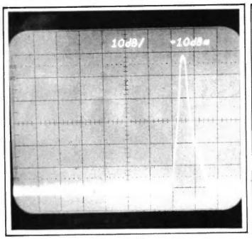
The RF bandpass at the mixer input (10dB/10MHz)
