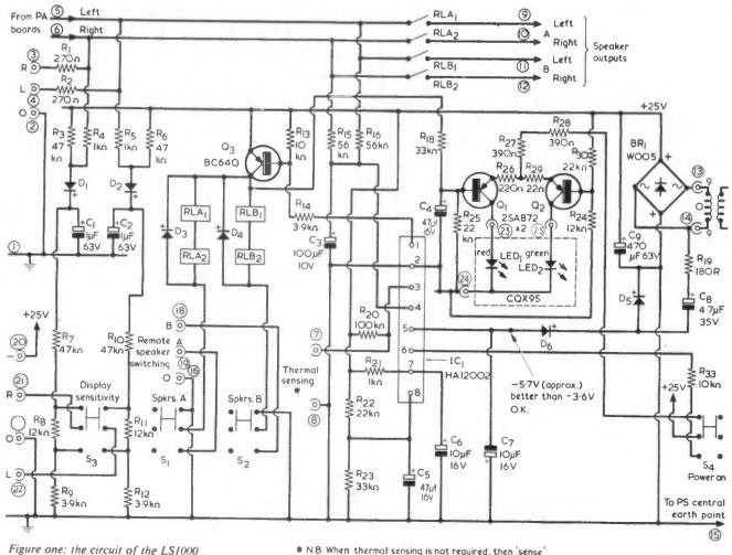
\* N.B. When thermal sensing is not required, then 'sense' pin must be shorted to ground (pin next to it)
