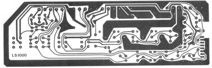
Figure two: Same size view of PCB foil side layout -
