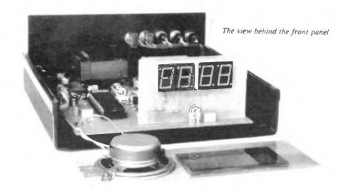
achieve the required memory vocabulary of about 20 words, as well as control, decoding and digital to analogue conversion, all on one MOS chip. Each word generated by the speech generator consists of a number of staircase-shaped pulses having a fixed period of 10 milliseconds. Each pulse is built up from 128 steps, and the smallest amplitude variation is 1/16th of the peak amplitude i.e. 4 bits of amplitude information.
