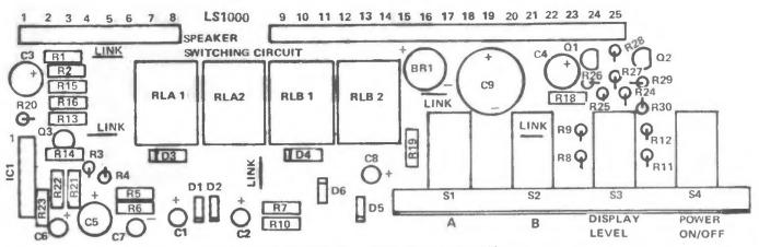
Figure three: The component overlay, superimposed on the PCB viewed from the component side.
