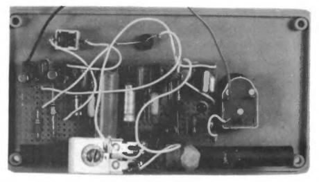
2. Internal view of the authors' Time Receiver. The circuit could be built into any nonmetallic enclosure.
