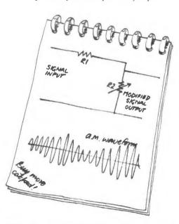
signal into a simple two resistor circuit. you get a fraction of the signal out of one of them."
