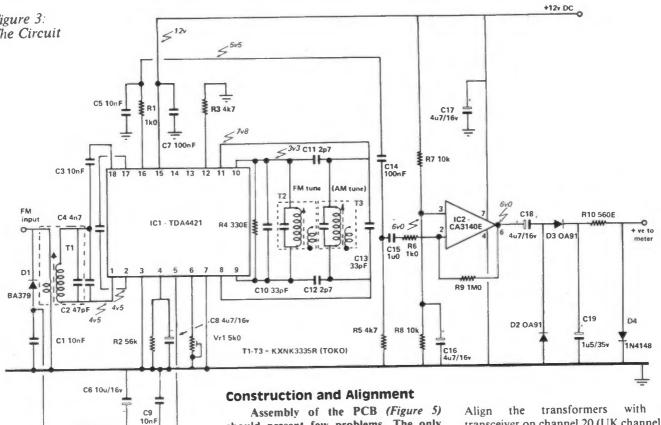
increases the dynamic range that the circuit will work over by some 30-40dB. centres the FM T2 Transformer demodulation 'S' curve on 27.8MHz (Figure 4).
