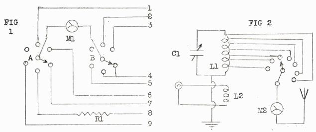
Fig 1 above shows the Meter and Function Switch circuit. The point connections are as follows: 1 to HT side BA anode; 2 to anode load side; 3 to top 100 ohms PA grid resistor; 4 to chassis; 5 toVFO anode load side; 6 to chassis; 7 to top PA cathode shunt; 8 to PA HT line; 9 to VFO anode HT side. R1 is a 100 K 1 watt multiplier which will make a 5mA 7 ohm meter read near enough 500 volts FSD. The spare position on switches A and B will eventually be used to read total current. M1 is 5 mA FSD.
