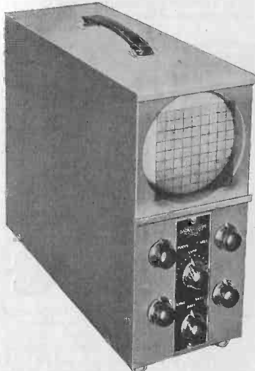
FIG. 8.—This Cossor Oscillograph is a useful example of the cathode-ray test apparatus.
