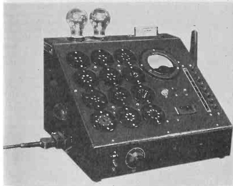
Fig. 12c. A Mullard Master Valve Tester (mains operated). Primarily designed for the testing of all types of valves; it has, however, numerous other applications.
