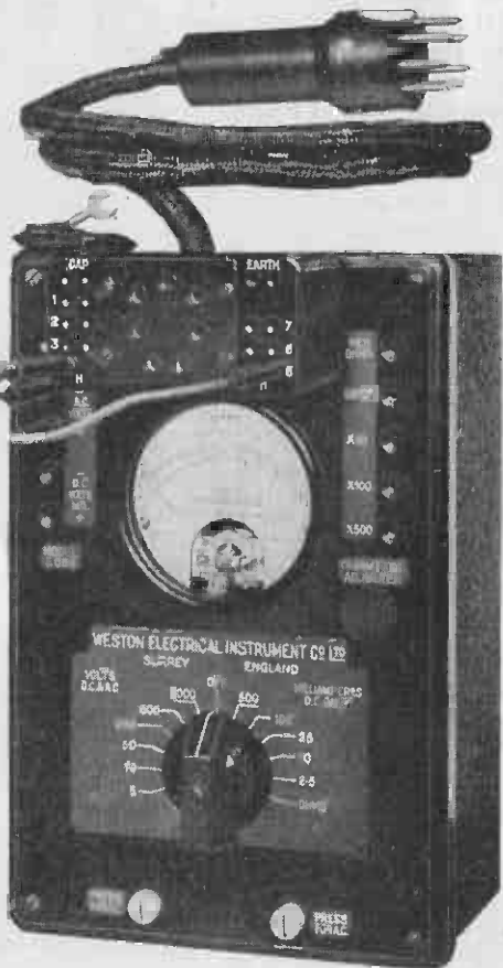
Fig. 6.—This is a typical set analyser, taken from the range of equipment supplied by the Weston Electrical Instrument Company.
