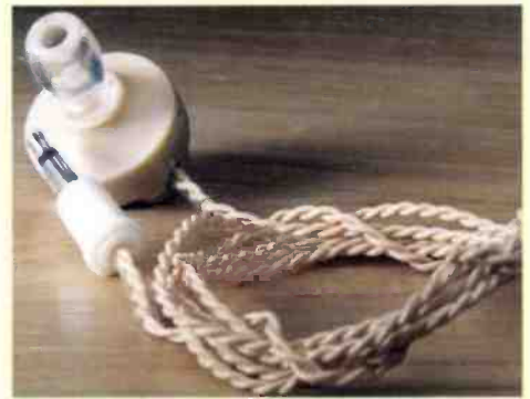
Fig. 4a: The design of this crystal earpiece hasn't changed in a long time.
