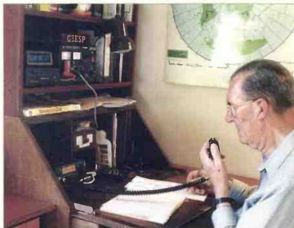
Pictured in 1997 in his shack, Walter G3ESP can be seen operating his Kenwood TS-50. Situated on the two shelves above is an AT-50 auto a.t.u. with a Watson p.s.u. to the right.
