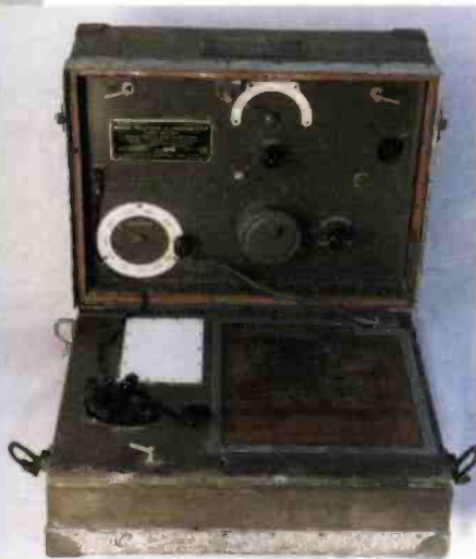
Fig. 1: Ben's 'junk shop' BC-148 transmitter-receiver. The set itself is housed in the lid of the box and the receiver batteries are under the Morse key. The chart mounted on the right of the Morse key is the unit's circuit diagram.
