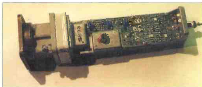
A microwave block being converted by Alan Kendall G6WJJ for use in the West Midlands 10GHz ATV repeater transmitter (see text).
