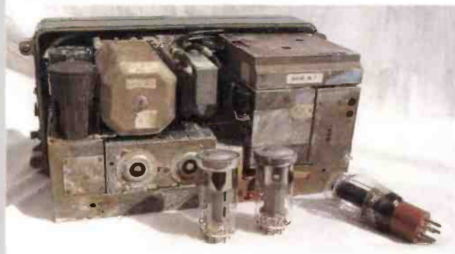
Fig. 5: Inside the Russian set. Note the modular construction. The 807 valve provides an indication of the size of the equipment and the Russian p.a. valve dimensions.
