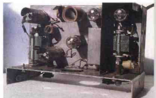
Fig. 7: Inside the Teco set with the receiver on the left, transmitter on the right. The modulator is in the centre and the p.a. stage tank coil at the top centre.
