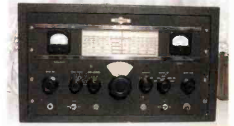
Fig. 2: The Collins 32V-1 transmitter clearly illustrating its very finely engineered tuning dial arrangement and symmetrical dial layout (see text).
