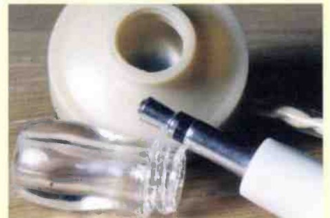
Fig. 4b: The diaphragm of the earpiece, mounted on the piezoelectric transducer, seen through the centre hole, is extremely fragile and shouldn't be touched.
