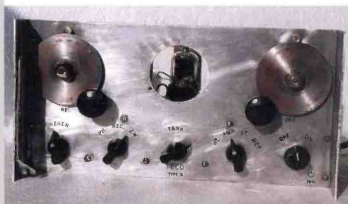
Fig. 6: The South African Teco wireless set (without meter). Note the very simple controls - the centre 'tank' knob tunes the p.a. stage (an 1Q5 valve). The date of manufacture (1941) is marked on a plate in the lower right-hand corner.
