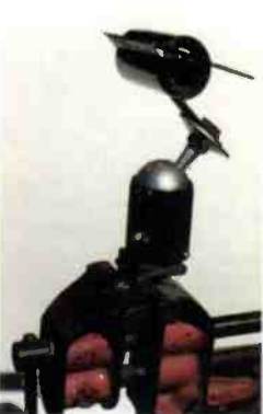
Fig. 5: A picture of John Olway's 'third hand' for holding p.c.b.s steady.
