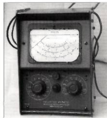
Fig. 2: A vacuum tube voltmeter (VTVM). The probe (illustrated in Fig. 1) is attached to this instrument. The photograph is of a valve voltmeter which I bought at a rally some years ago. It's a Marconi type TF 1041C, manufactured in 1962.
