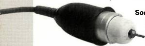
Fig. 1: A diode r.f. probe (see text).
