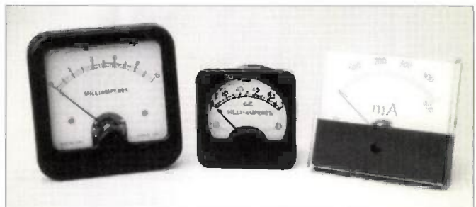
Fig. 5: A selection of useful surplus moving coil milliammeter (see text).
