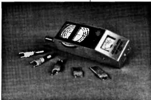
Fig. 4: A dip meter, whether valved or transistorised, can be useful in many ways in an amateur radio workshop. Many operators even use them as simple signal generators.
