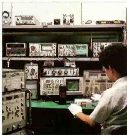
Final quality checks on an MVT-8000.
