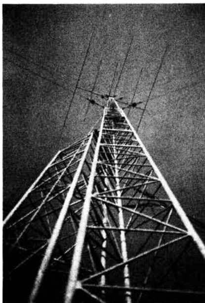
My home-brew 3-element Yagi for 14MHz and the Elan for 21/28MHz
