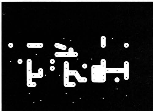
Fig. 2.2: Double-sided track pattern (shown full size) and component overlay of oscillator module
