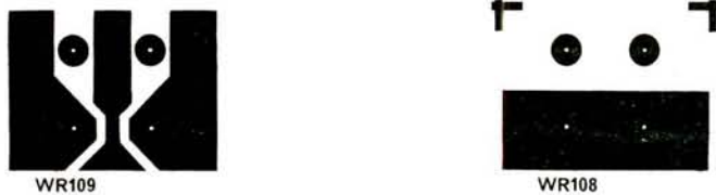
Fig. 17: The end cheeks of the transformers. One of each of the p.c.b.s shown here are required for each transformer. The brass tubes must be soldered to the copper pads which are on the outer ends of the transformers. The material is 3mm copper-clad board
