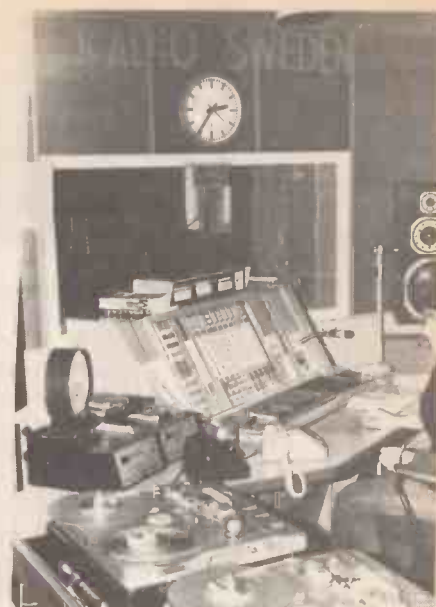
Continuity suite for Radio Sweden. The cartridge machine on the left provides multi-lingual station identifications
